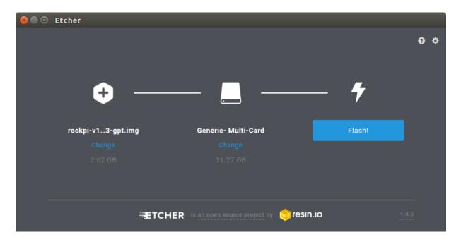
In the etcher window, once it shows us Flash Complete! It is done and can be put into the ROCK Pi S.
