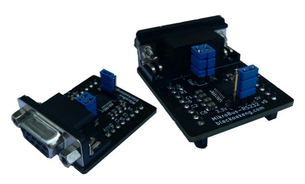
*Description.* Many electronic devices expose the UART only as logic (TTL) levels. In order to interface with a traditional RS232 port, the signals must be converted to higher, bipolar voltages. That's what the MikroBus-RS232 does. It uses the industry standard MikroBus footprint. It also has shunts to change from Normal operation to Null modem. The RS232 connector is a standard DSub-9.
