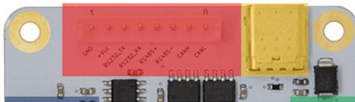
Figure 3: Power / communication connector of TMCM-0960-MotionPy V21
