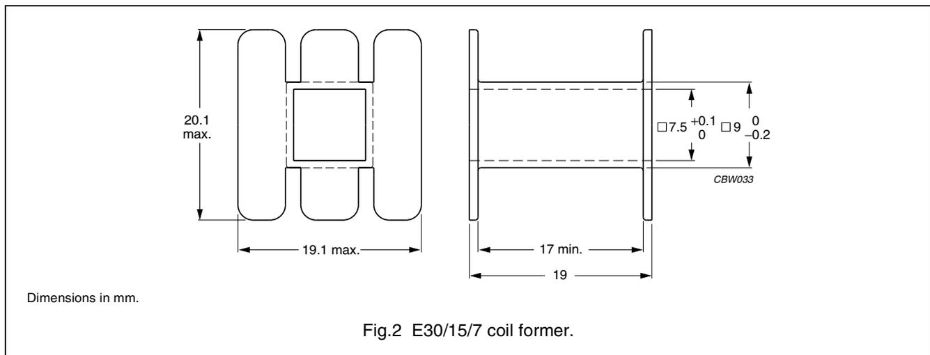
**WINDING DATA AND AREA PRODUCT FOR E30/15/7 COIL FORMER WITHOUT PINS (E)**
