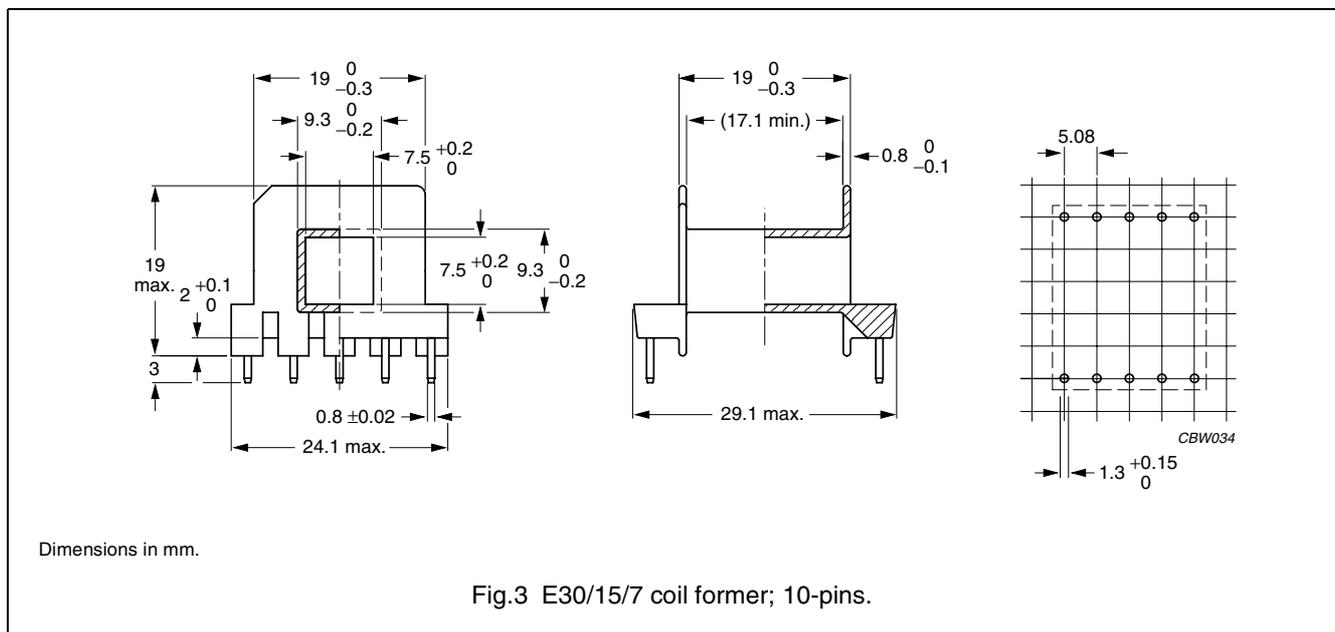
**WINDING DATA AND AREA PRODUCT FOR 10-PINS E30/15/7 COIL FORMER (E)**
