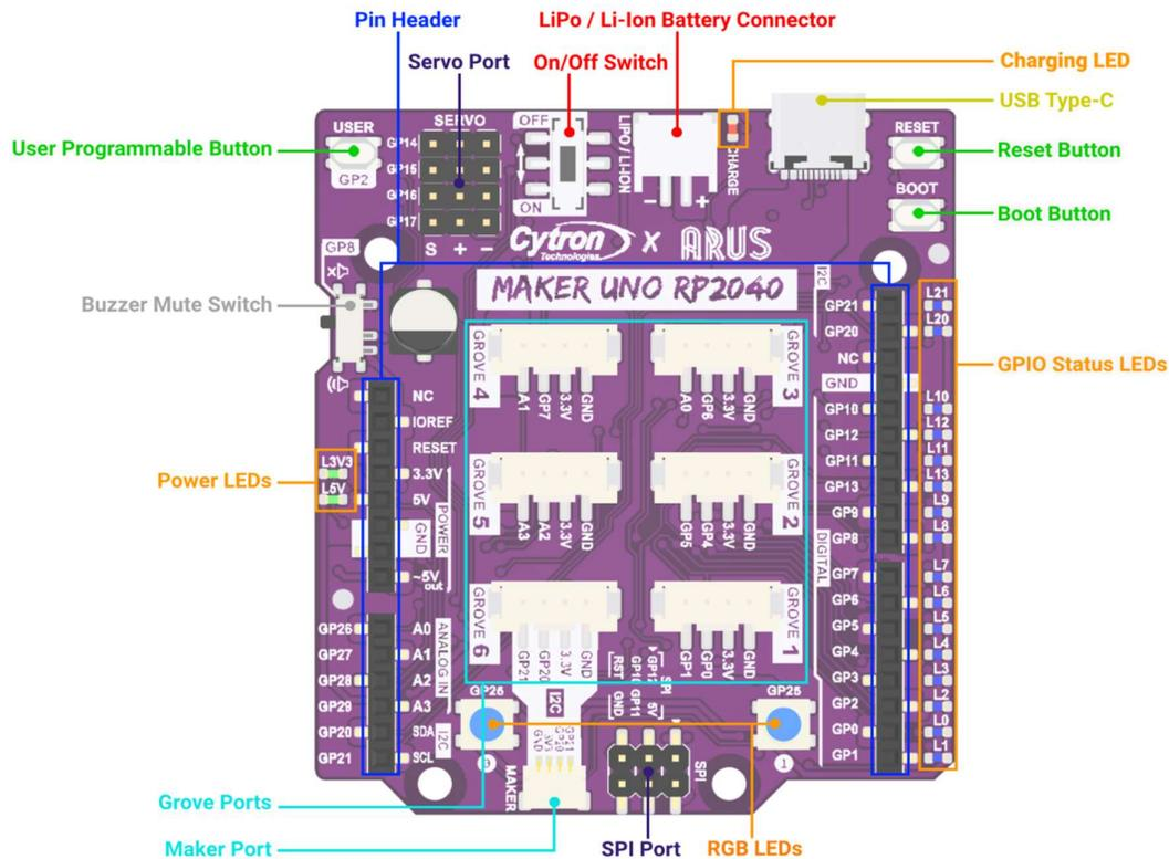
Figure 1: MAKER-UNO-RP2040 Board Functions (TOP)
