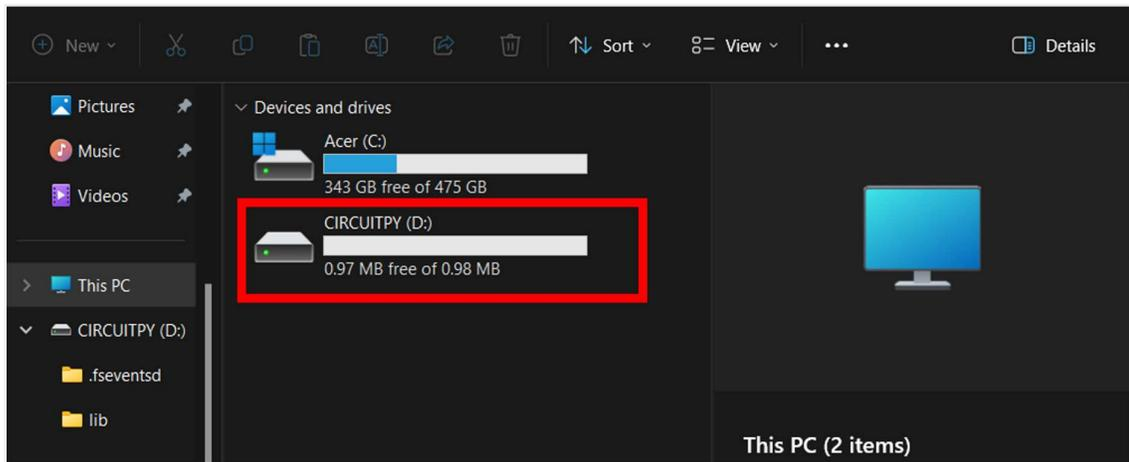
3. Now let's try a simple code to verify that everything is working correctly. At the bottom right corner of the window make sure the correct Configure Interpreter, **CircuitPython (generic)** and COM are shown and chosen.
