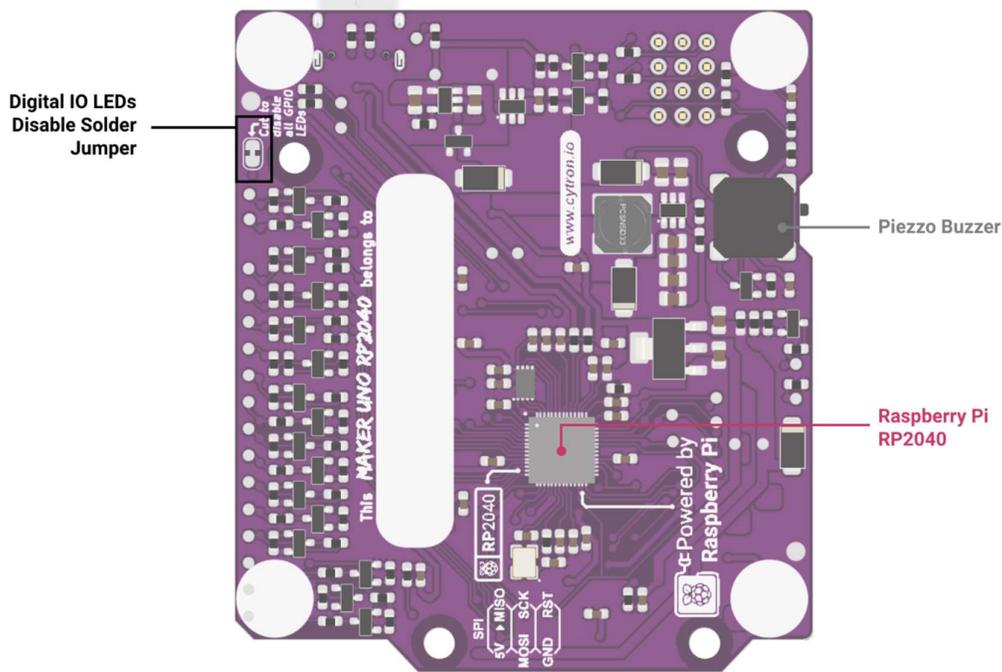
Figure 2: MAKER-UNO-RP2040 Board Functions (Bottom)
