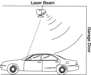
5. When your car first enters the garage, the motion detector will turn on the laser. Drive forward until the laser beam hits your pre-determined spot indicating that you are parked in the correct position. The laser will turn off automatically after you are parked.
