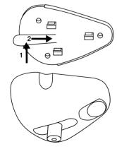
3. Mount the unit close to an electrical outlet (typically near the one used to power your garage door opener). Plug in the AC adapter. The battery is only a backup if power is interrupted and will not last for more than a few days. To install the backup battery, remove the screw on the rectangular battery compartment on top of the main unit.
