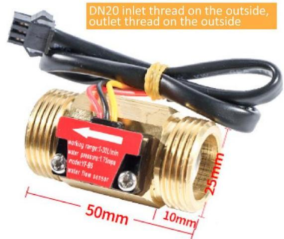
Water flow sensor consists of a copper body, a water rotor, and a hall-effect sensor. When water flows through the rotor, rotor rolls. Its speed changes with different rate of flow. The hall-effect sensor outputs the corresponding pulse signal. This one is suitable to detect flow in water dispenser or coffee machine.
