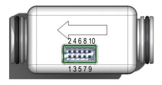
The SFM3100 is designed for connector attachment and uses Molex Milli-Grid 87831-1041 (THT). Please refer to the datasheet of this part for mating connectors.
