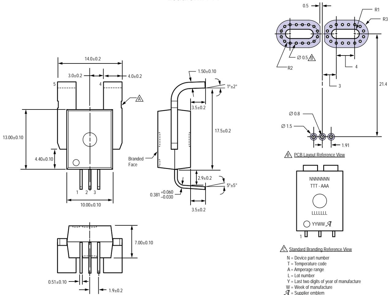
Creepage distance, current terminals to sensor pins: 7.25 mm
