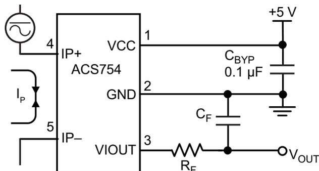
Application 1. The ACS754 outputs an analog signal,  $V_{OUT}$ , that varies linearly with the uni- or bi-directional AC or DC primary sensed current,  $I_P$ , within the range specified.  $C_F$  is recommended for noise management, with values that depend on the application.
