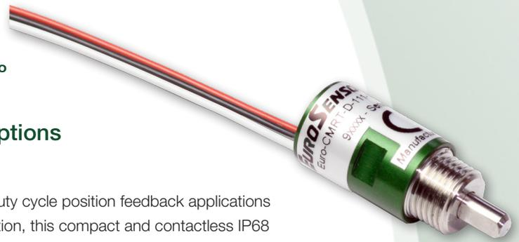
The Euro-CMRT angle sensor is specifically aimed at arduous high-duty cycle position feedback applications where miniaturisation is a key factor. With programmable angle selection, this compact and contactless IP68 rated Hall Effect sensor features a high grade aluminium housing and a stainless steel shaft which together with the M8 mounting thread are all customisable to suit the customer's application.
