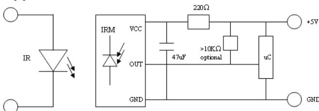
RC Filter should be connected closely between Vcc pin and GND pin.
