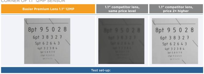
Camera: acA4112-20um (sensor: 12MP – IMX 304, pixel size 3.45 μm)
