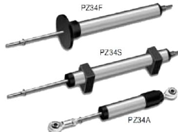
This mini position transducer is designed for direct absolute measurement and available in stroke length up to 250 mm. The mini design is suitable for mounting in instruments or machines with limited space. An improved technique for making a connection to the resistance track (Double Trimming Technique) ensures the higher degrees of reliability and linearity, while multi-fingers wipers stabilize output signals, even in the most adverse working conditions.
