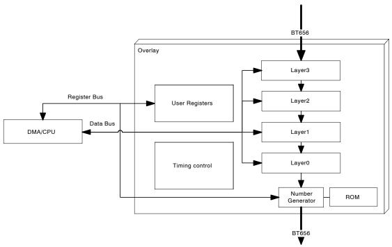
Figure 26. Internal Block Diagram Overlay
