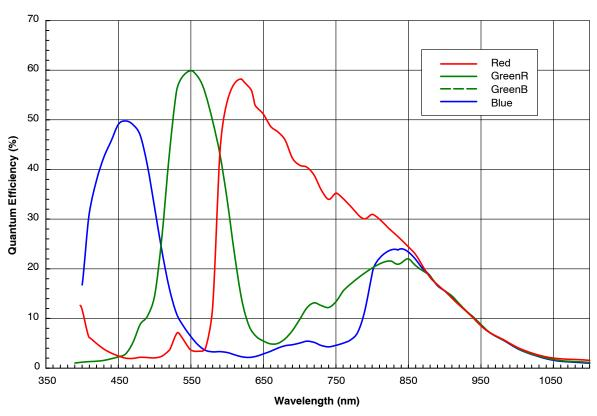
NOTE: The measurements were done on packaged parts with regular glass coating (that is, without Anti–Reflective Glass (ARC) coating).
