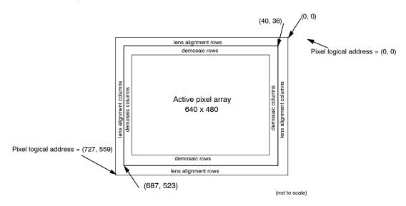
Figure 5. Pixel Array Description
