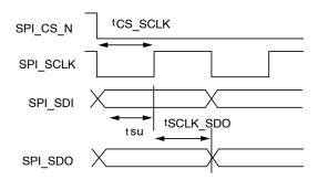
Figure 45. SPI Output Timing
