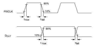
Figure 37. Slew Rate Timing
