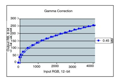
Figure 11. Gamma Correction Curve
