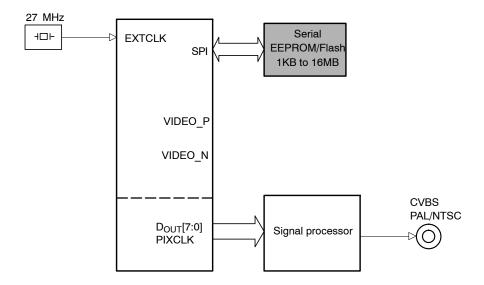
Figure 13. External Signal Processing Block Diagram
