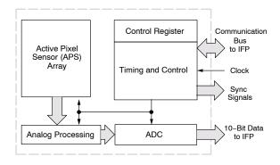
Figure 4. Sensor Core Block Diagram
