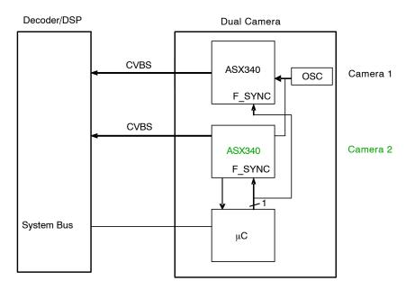
Figure 12. Multicamera System Block Diagram
