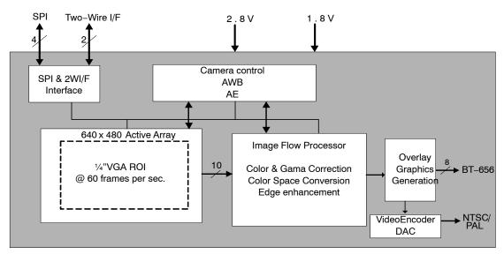
Figure 2. Internal Block Diagram
