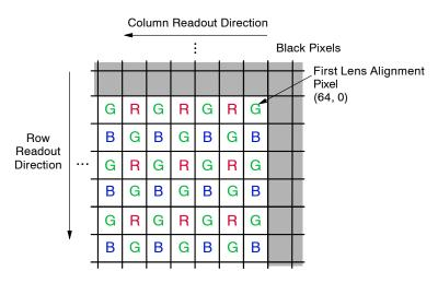
Figure 7. Pixel Color Pattern Detail (Top Right Corner)
