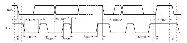
Figure 49. Two-Wire Serial Bus Timing Parameters
