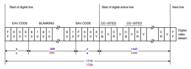
Figure 29. CCIR656 8-Bit Parallel Interface Format for 525/60 (625/50) Video Systems
