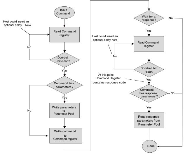
Figure 16. Host Command Process Flow
