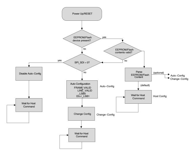
Figure 14. Power-Up Sequence - Configuration Options Flow Chart
