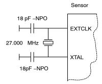
NOTE: Value of load capacitor is crystal dependent. Crystal with small load capacitor is recommended.
