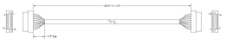
One Meter Cable Both Ends Terminated: 2080AG039 = 14 conductor 28 AWG for differential UVW Commutation 2094AG039 = 11 conductor 28 AWG for single-ended UVW Commutation (TTL or open collector) 2082AG039 = 8 conductor 28 AWG for non-Commutation *Connector = JAE FI-W15S*
