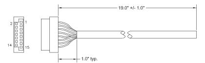
Half Meter Cable One End Terminated: 2081AG019 = 14 conductor 28 AWG for differential UVW Commutation 2095AG019 = 11 conductor 28 AWG for single-ended UVW Commutation (TTL or open collector) 2083AG019 = 8 conductor 28 AWG for non-Commutation
