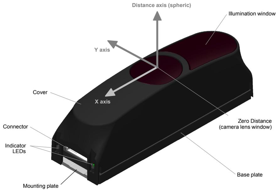
Figure 3: Mechanical features
