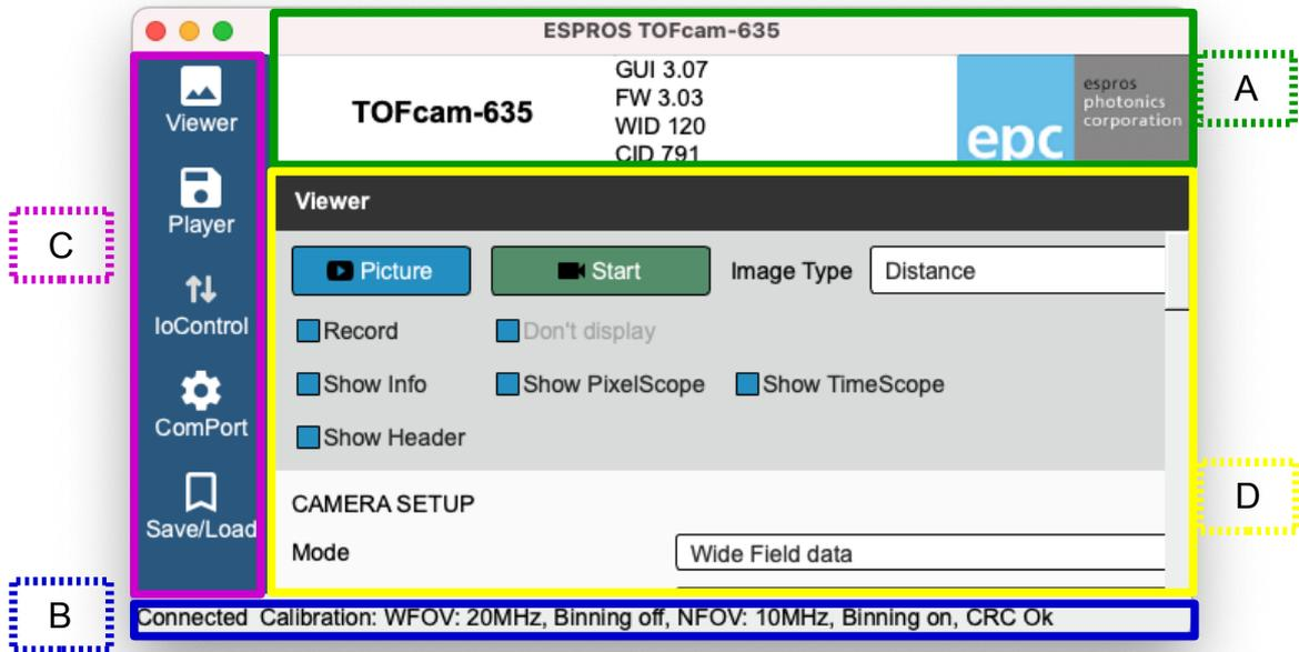
Figure 11: Sections of the GUI main screen
