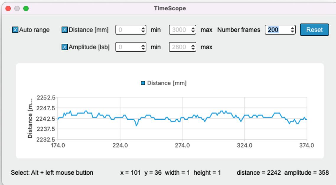
Figure 27: Timescope
