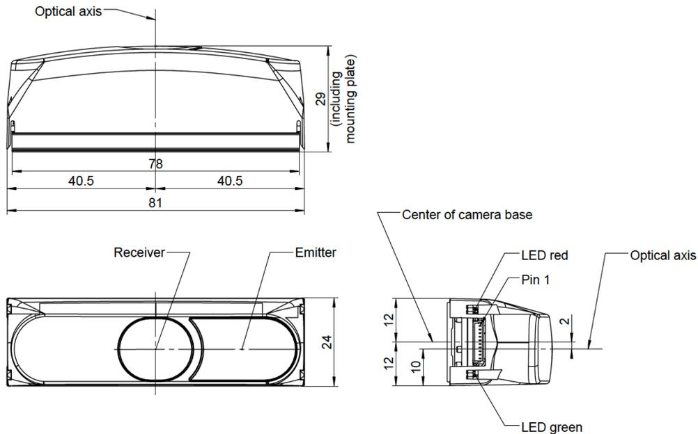
Figure 4: Mechanical dimensions
