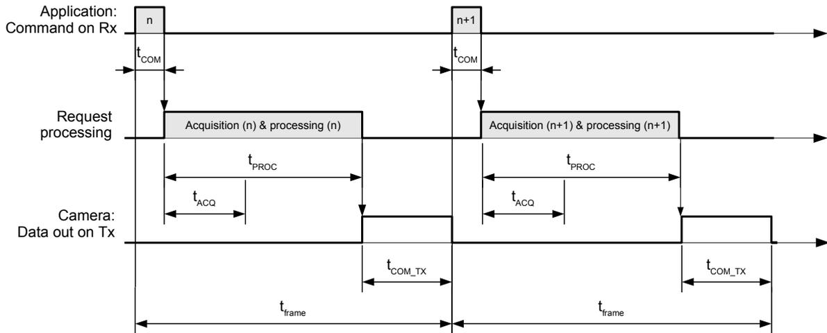
Figure 41: Timing of a single distance measurement
