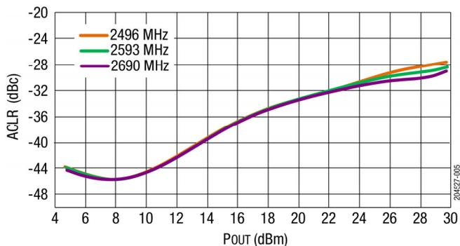
Figure 5. LTE 5x20 MHz ACLR1 vs Pout Across Frequency
