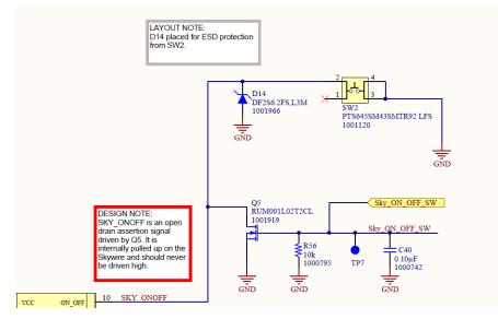
To conserve power, the onboard cellular module does not automatically startup when power is applied. The baseboard design must supply a means to assert a logic-low level on the ON\_OFF pin. To initiate the startup procedure, tie ON\_OFF to ground for at least 500 ms.
