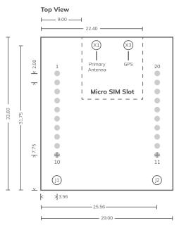
When using soldering directly to a PCB, ensure that any baseboard components placed under the Skywire (between the baseboard header pin connectors) are no taller than 0.5 mm.
