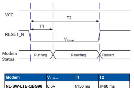
If the signal is unused, it can be left floating, but it is highly recommended that the signal be connected to the host system. If the signal is used, it should be driven with an open collector output from the host system or a discrete open collector transistor.
