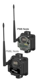
The Sure Cross® wireless system is a radio frequency network with integrated I/O that operates in most environments to eliminate the need for wiring runs.
