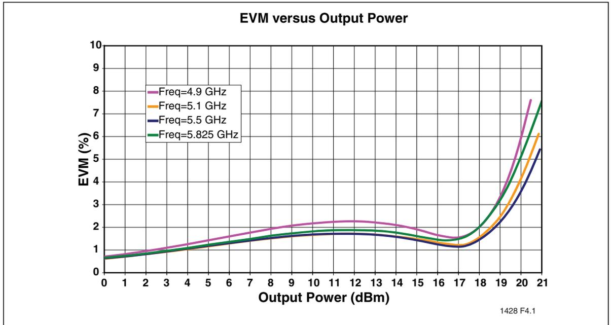
Figure 3: EVM versus Output Power,  $V_{CC} = 3.3V$ ,  $V_{REG} = 2.85$
