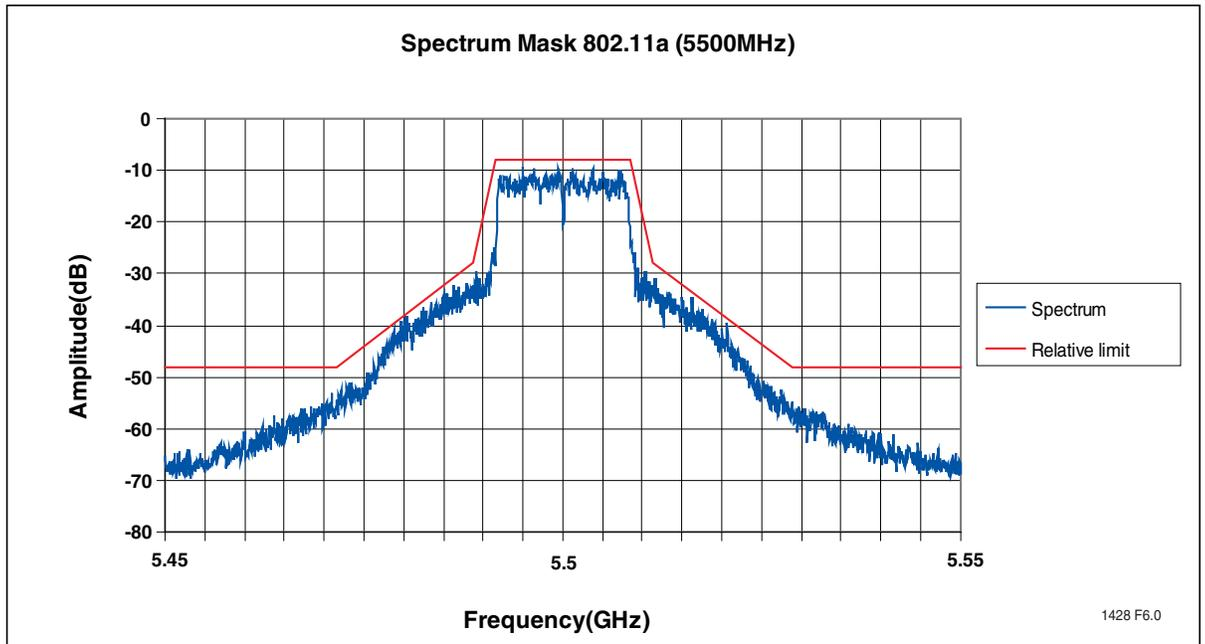
**Figure 6:** Maximum Mask Compliance,  $V_{CC} = 3.3V$ ,  $V_{REG} = 2.85$ , Frequency = 5.5 GHz at  $P_{OUT} = 23.3$  dBm with  $I_{CC} = 390$  mA
