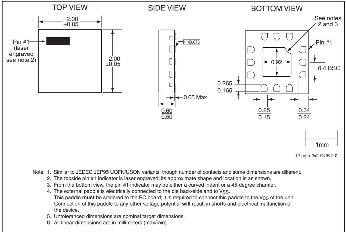
**Figure 15:** 12-contact Ultra-thin Quad Flat No-lead (UQFN)
