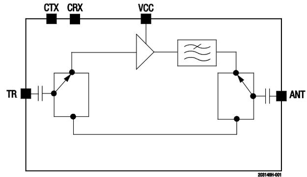
**Figure 1. SKY66110-11 Functional Block Diagram**
