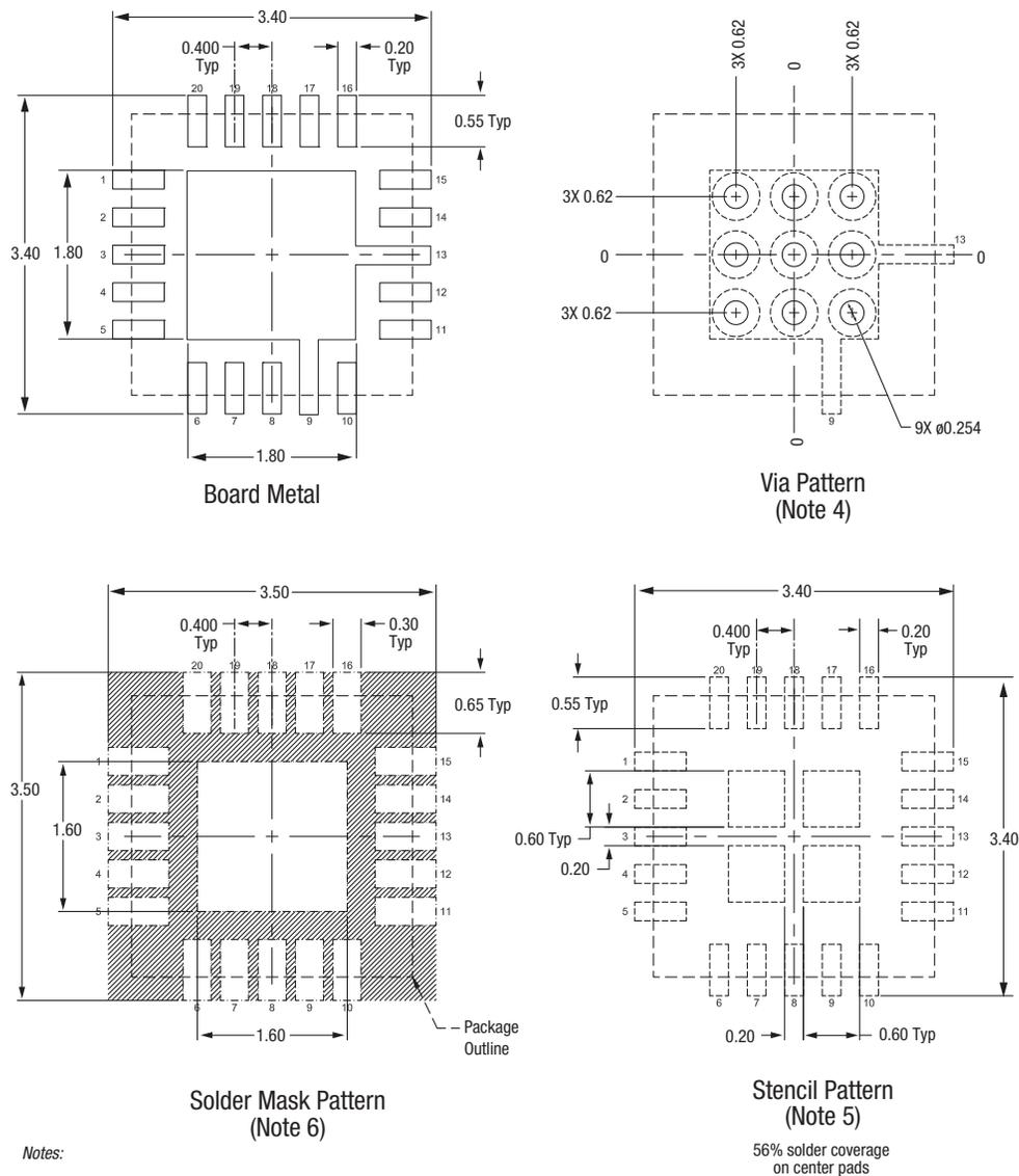
Figure 4. PCB Layout Footprint for the SE2611T
