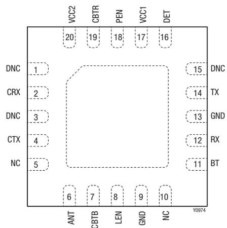
**Figure 1. SE2611T Pinout – 20-Pin QFN (Top View)**
