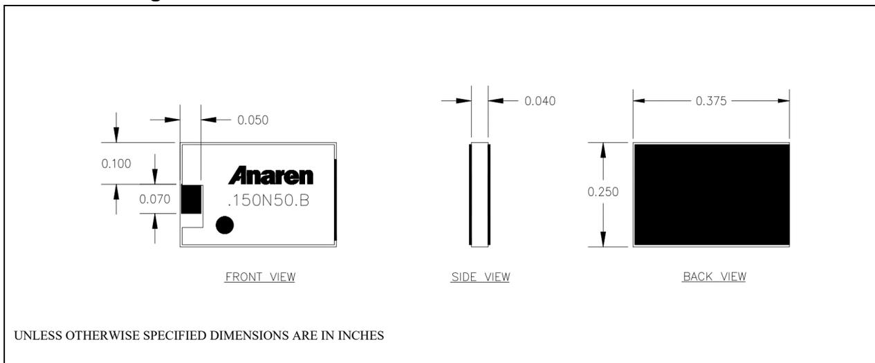
Tolerance is ±0.010", unless otherwise specified. Designed to meet or exceed applicable portions of MIL-E-5400. All dimensions in inches.
