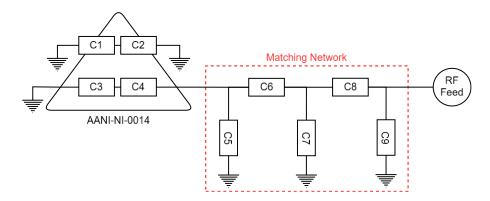
However, it is common that the resonant frequency will shift during implementation in an arbitrary device. Therefore, this matching may be changed with other values/components/brands for compensation of such effects. This is further described in the General Implementation Guidelines section below.
