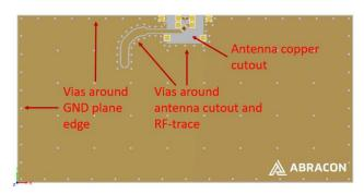
The rectangular copper cutout in the footprint needs to go through all the layers in the PCB stackup, meaning that there cannot be copper on any layer in this area. It is also recommended to have a good via-structure around the cutout and the edge of the ground plane, see the right image above.
