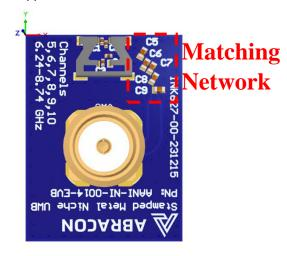
The evaluation board has a matching circuit implemented next to the antenna to enable optimization possibilities for the user. The C1-C4 component footprints are sized for 0201 (0603 metric) SMD components. The matching network (C5-C9) component footprints are sized for 0402 (1005 metric) SMD components.
