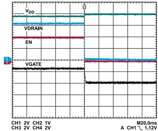
Figure 58. Turn Off HMC980LP4E Outputs to ADPA7005CHIP
