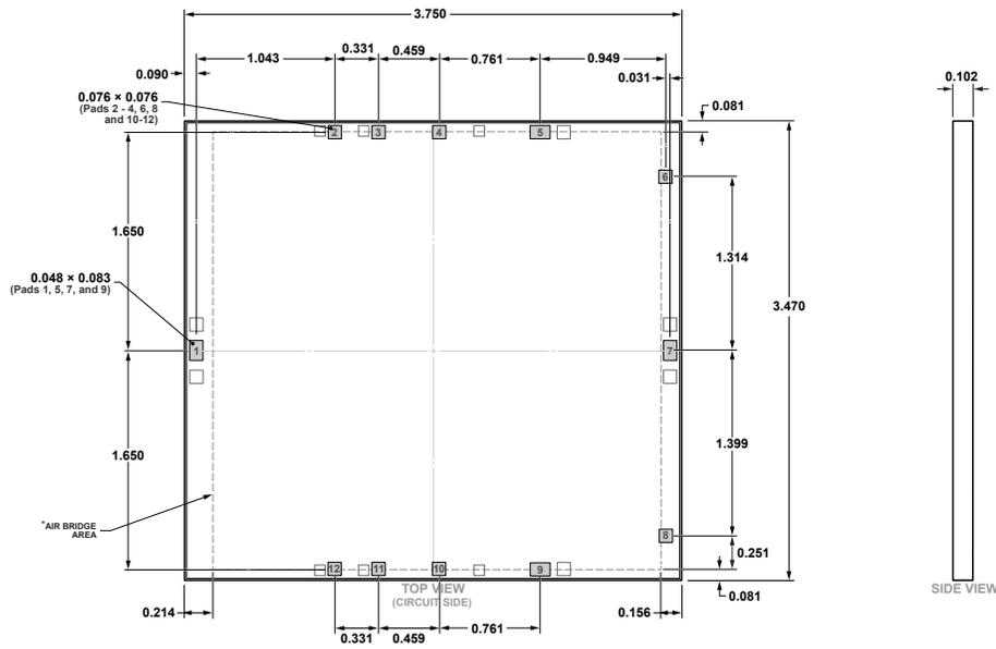
\*This die utilizes fragile air bridges. Any pickup tools used must not contact this area.
