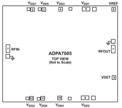
Figure 2. Pin Configuration
