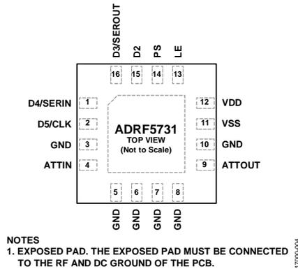
Figure 4. Pin Configuration
