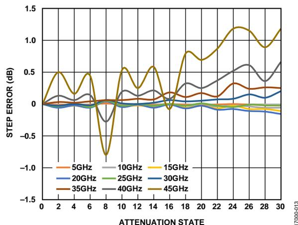
Figure 15. Step Error vs. Attenuation State over Frequency
