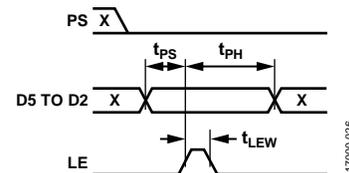
Figure 27. Latched Parallel Mode Timing Diagram
