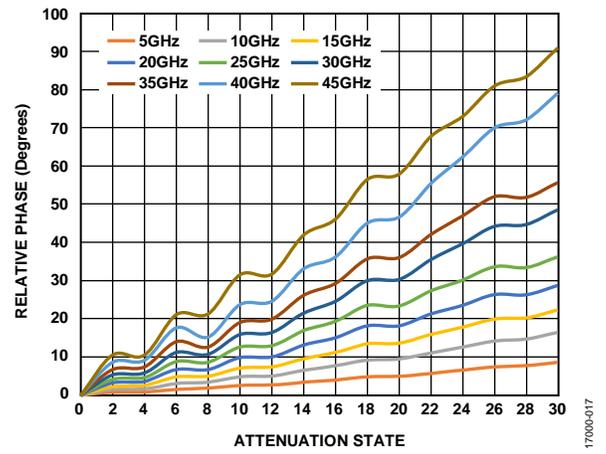
Figure 19. Relative Phase vs. Attenuation State over Frequency
