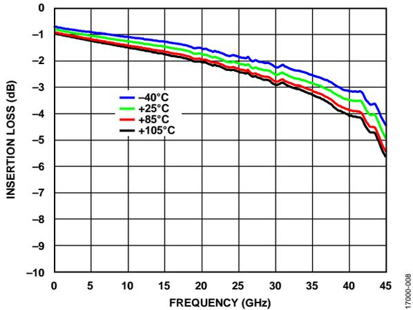
Figure 10. Insertion Loss vs. Frequency over Temperature
