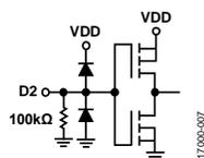
Figure 6. Digital Input Interface Schematic for D2
