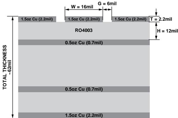
Figure 28. Evaluation Board Stackup, Cross Sectional View
