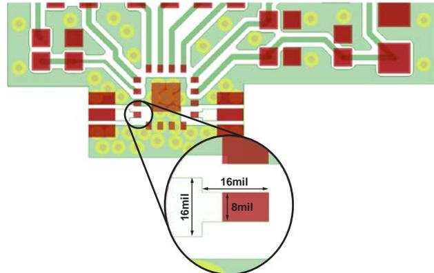
Figure 34. Probe Board Layout Dimensions (Top View)
