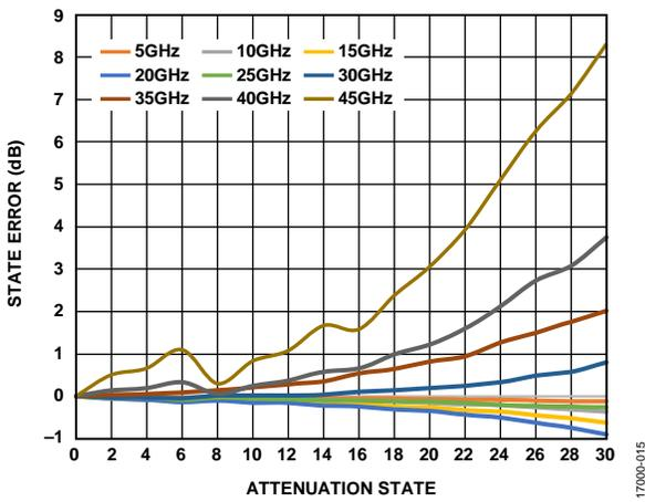
Figure 17. State Error vs. Attenuation State over Frequency
