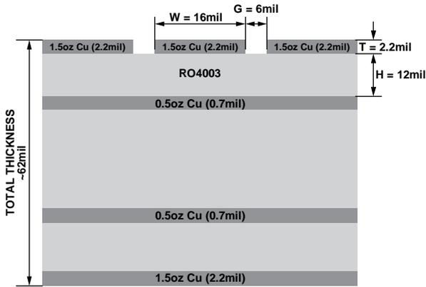
Figure 32. Probe Matrix Board (Cross Sectional View)
