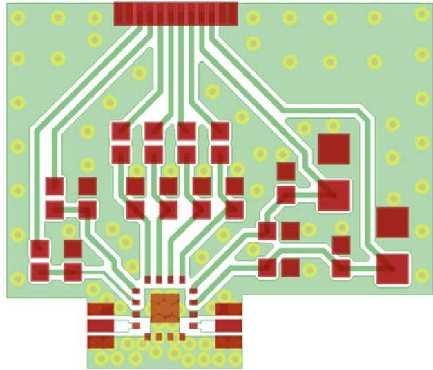
Figure 33. Probe Matrix Board Layout (Top View)
