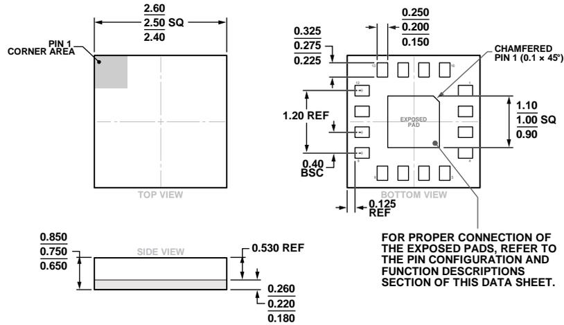
Figure 35. 16-Terminal Land Grid Array [LGA]
