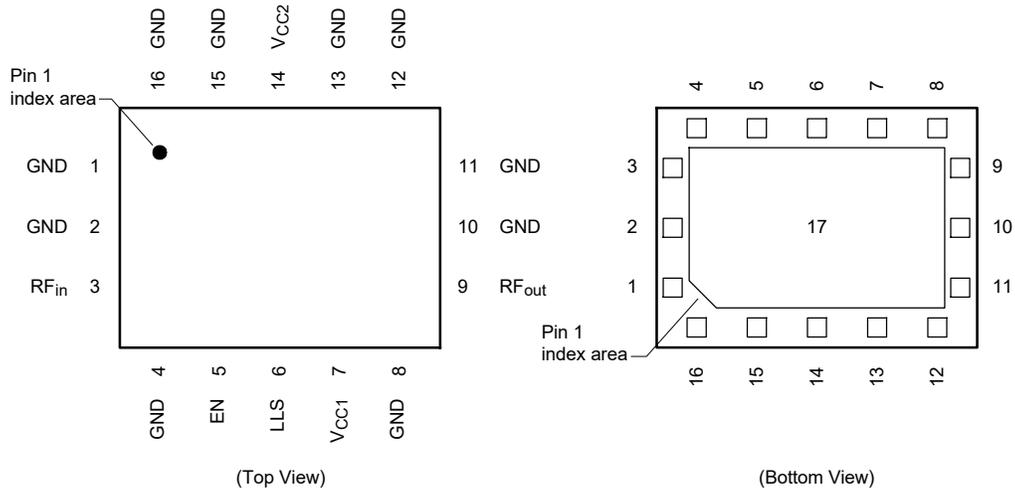
**Figure 2. Pin Connections**
