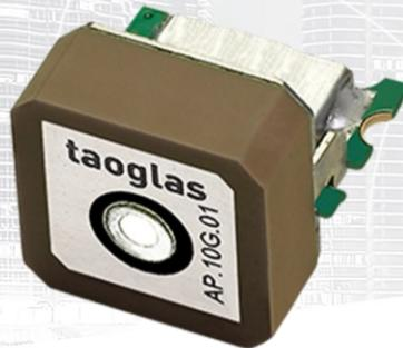
The AP.10G.01 one stage 14dB active GPS/Galileo patch antenna is the smallest SMD GPS/Galileo high performance embedded antenna currently available in the world. Using extremely sensitive high dielectric constant powder formulation and tight process control the 10mm x 10mm x 4mm patch antenna is accurately tuned to have its frequency band right at 1575.42MHz for GPS/Galileo systems.
