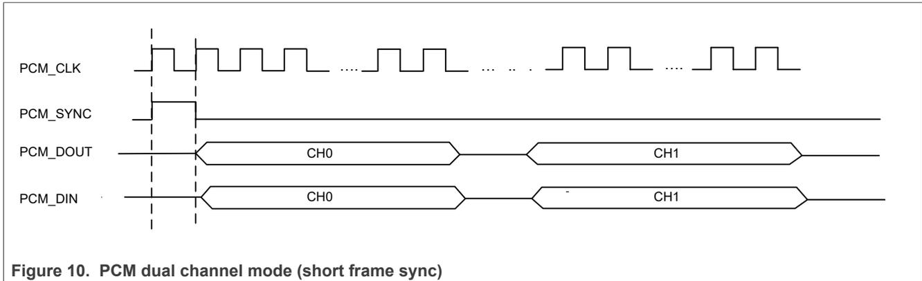
Figure 10. PCM dual channel mode (short frame sync)
