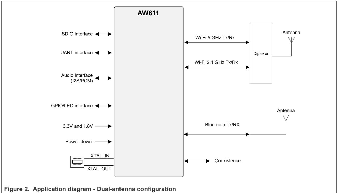
Figure 2. Application diagram - Dual-antenna configuration
