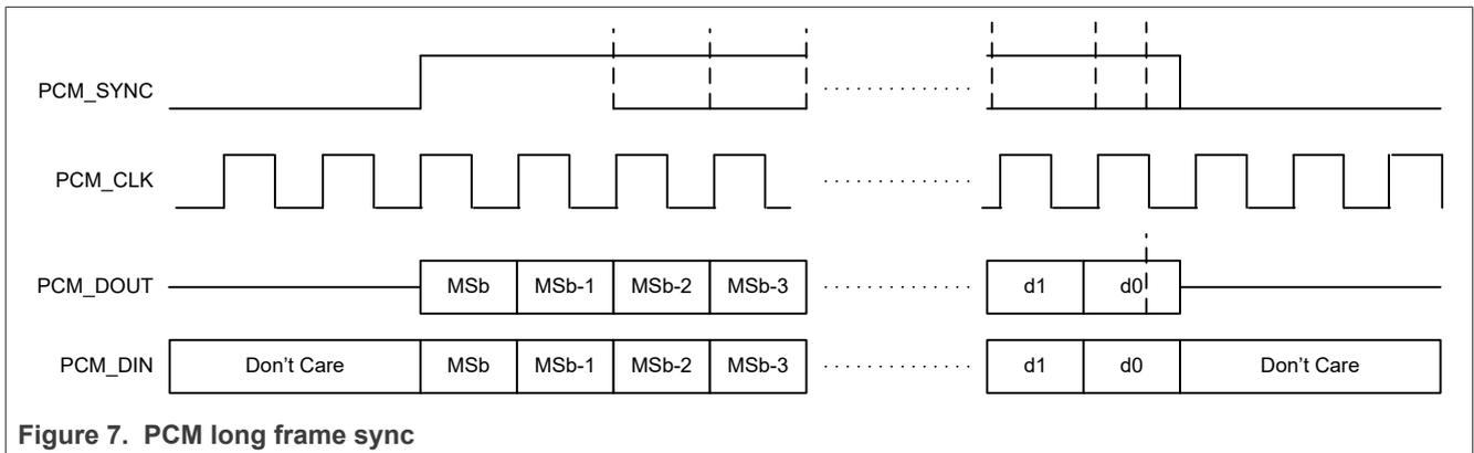
Figure 7. PCM long frame sync
