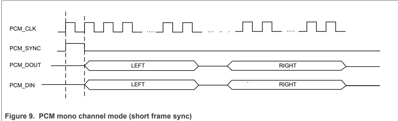
Figure 9. PCM mono channel mode (short frame sync)
