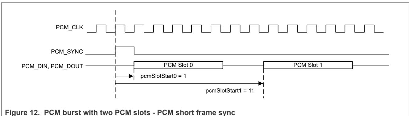
Figure 12. PCM burst with two PCM slots - PCM short frame sync
