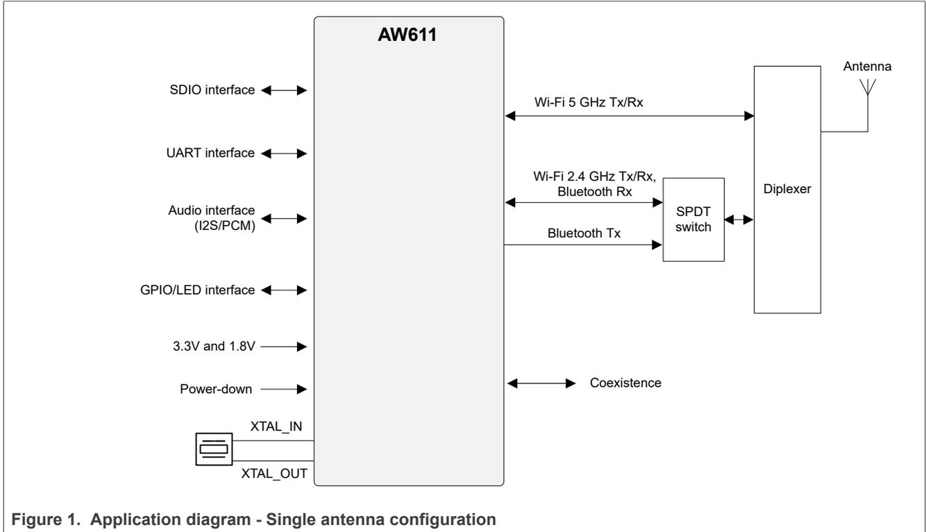
Figure 1. Application diagram - Single antenna configuration
