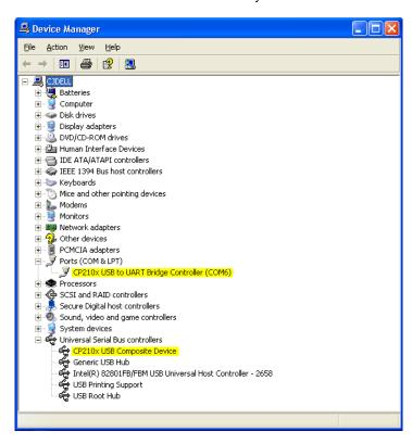
The CP2102 chip provides the functionality to use standard UART serial communications from your computer via the Universal Serial Bus, and interfaces directly to our Bluetooth module inside the BT233/224 Bluetooth serial adapter.
