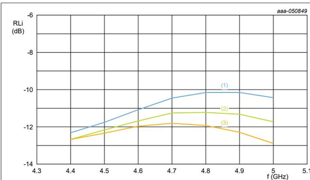
Figure 9.  $RL_i$  versus frequency over temperature
