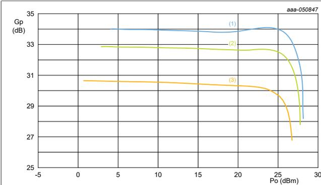
Figure 7. Gain versus  $P_{out}$  over temperature at 5 GHz
