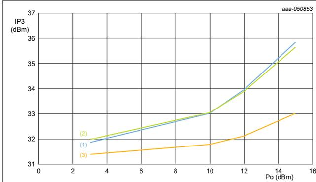
**Figure 13. IP3 versus  $P_{out}$  over temperature at 4.4 GHz**
