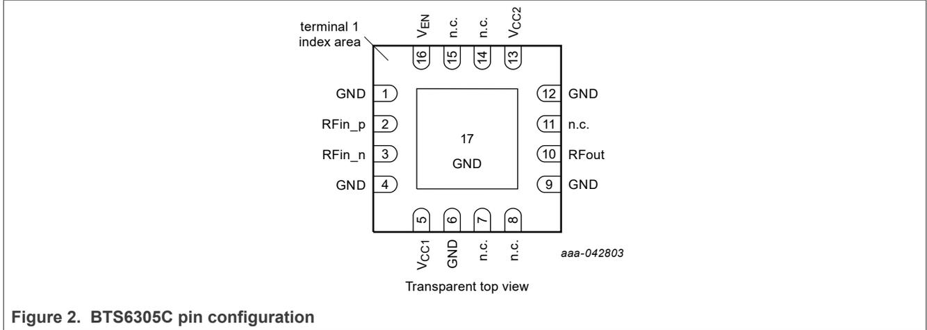
Figure 2. BTS6305C pin configuration
