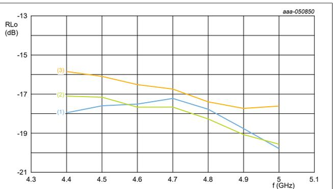
Figure 10.  $RL_o$  versus frequency over temperature
