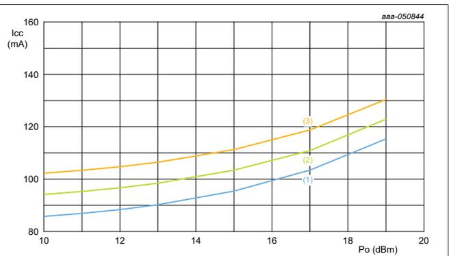
**Figure 4.  $I_{CC}$  versus  $P_{out}$  over temperature at 4.4 GHz**
