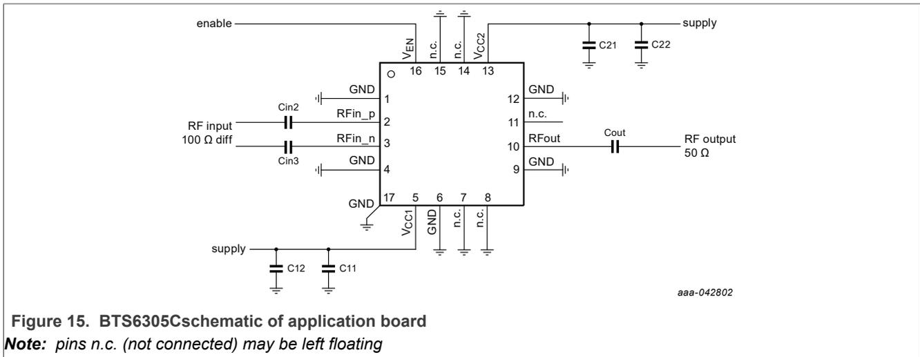
**Figure 15. BTS6305Cschematic of application board**
