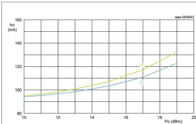
**Figure 3.  $I_{CC}$  versus  $P_{out}$  over frequency at  $25\text{ }^{\circ}\text{C}$**
