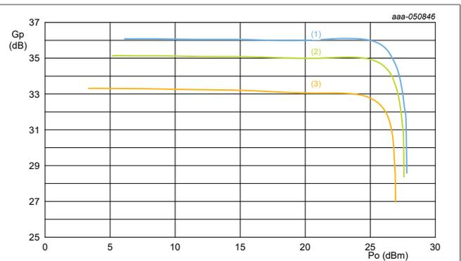
**Figure 6. Gain versus  $P_{out}$  over temperature at 4.4 GHz**
