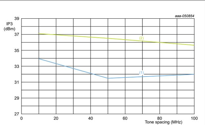
**Figure 14. IP3 versus Tone spacing over  $P_{out}$**
