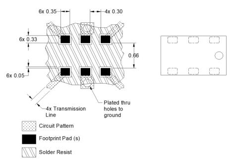
Dimensions are in Millimeters Mounting Footprint
