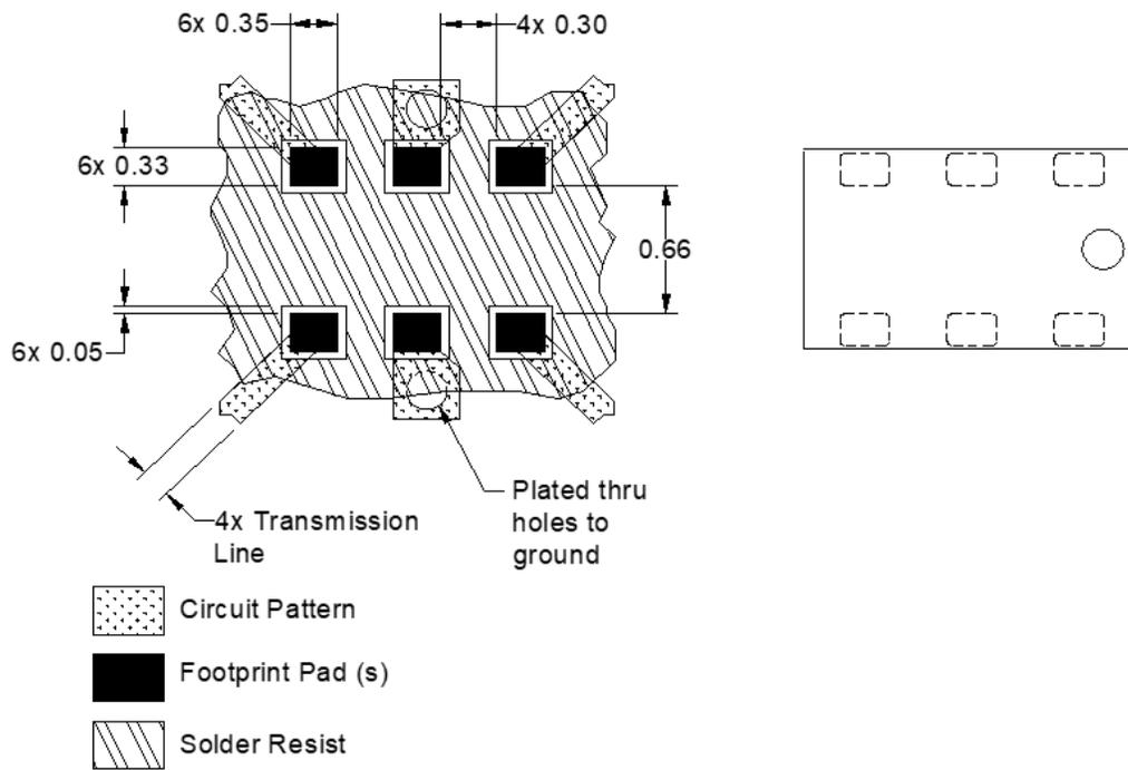
Dimensions are in Millimeters
