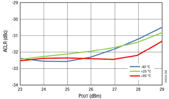
Figure 6. ACLR2 (2x20 MHz) vs Pout Across Temperature
