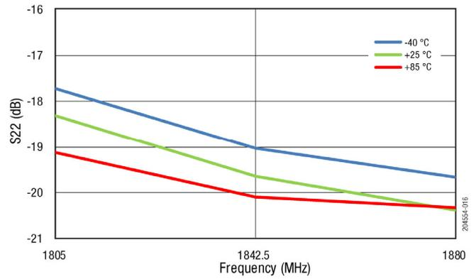
**Figure 16. S22 vs Frequency Across Temperature (P<sub>IN</sub> = -20 dBm)**
