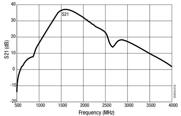
Figure 14. Wide Band Small Signal Gain vs Frequency
