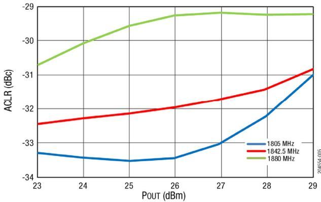
Figure 5. ACLR2 (2x20 MHz) vs. Pout Across Frequency
