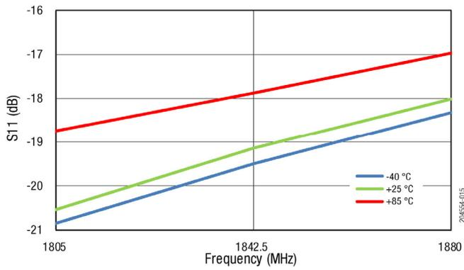
**Figure 15. S11 vs Frequency Across Temperature (P<sub>IN</sub> = -20 dBm)**
