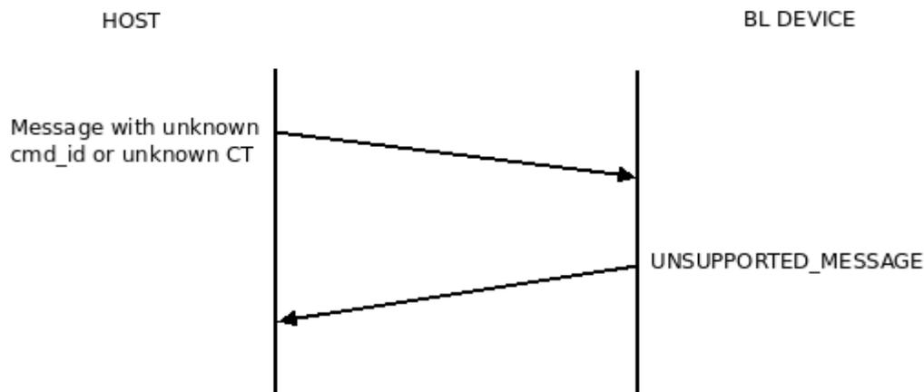
**Figure 4. Unsupported data received by BL Device**
