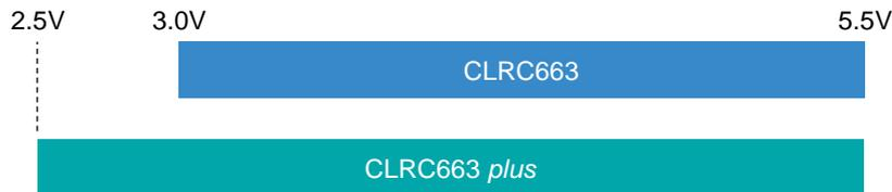
CLRC663 *plus* enables better support for battery powered systems
