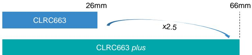
CLRC663 *plus* has new configuration options<sup>(2)</sup> enabling up-to 2.5x the detection range in LPCD<sup>(1)</sup> mode
