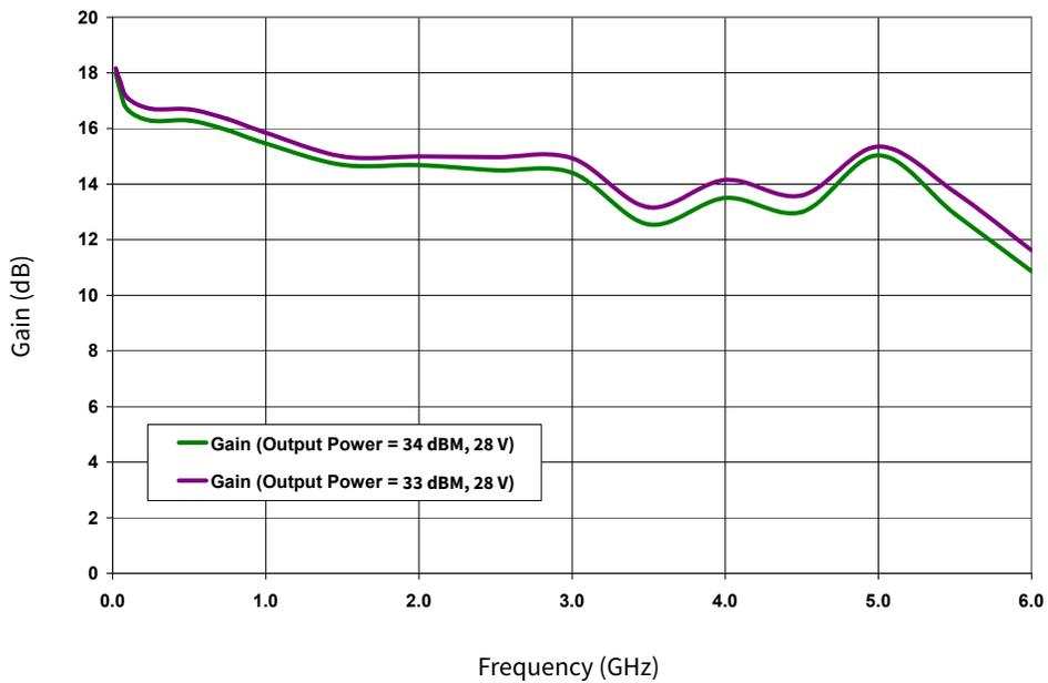
Figure 2. Power Gain vs Frequency at 28 V
