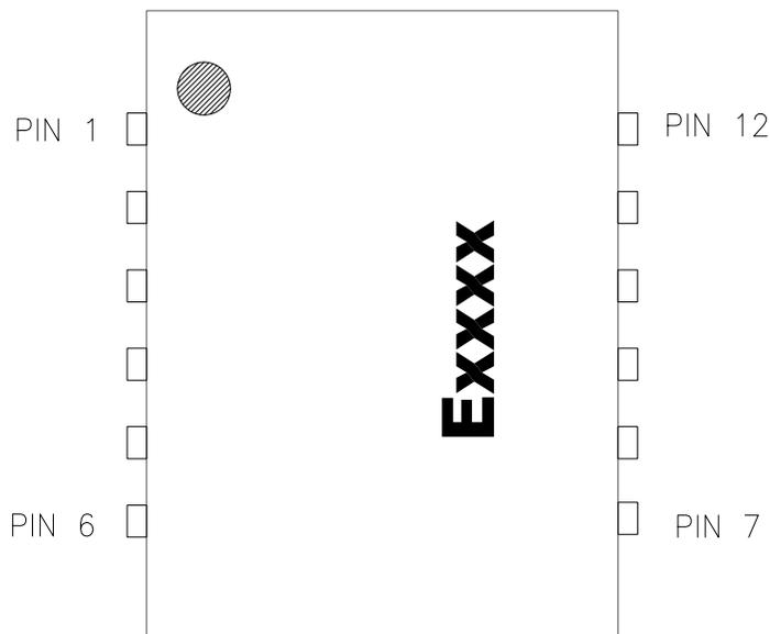
Note: Leadframe finish for 3x4 DFN package is Nickel/Palladium/Gold. Gold is the outer layer
