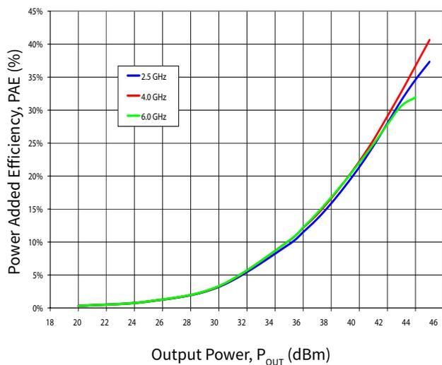
Figure 6. Power Added Efficiency vs Output Power as a Function of Frequency
