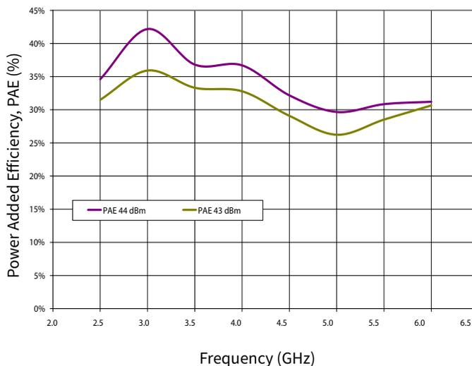
Figure 7. PAE at 43 dBm and 44 dBm Output Power vs Frequency
