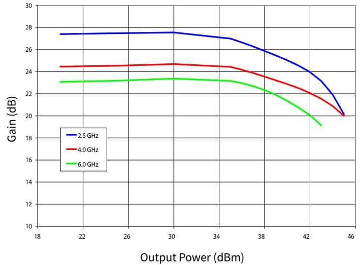
Figure 4. Gain vs Output Power as a Function of Frequency
