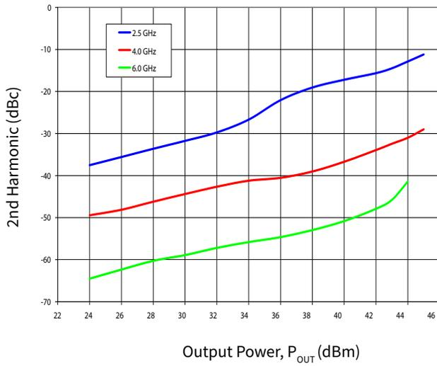
Figure 8. 2nd Harmonic vs Output Power as a Function of Frequency
