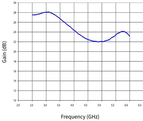
Figure 1. Small Signal Gain vs Frequency
