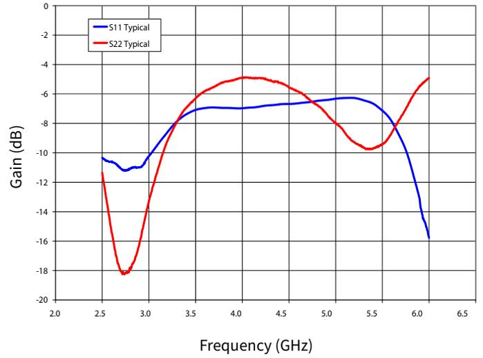
Figure 2. Input & Output Return Losses vs Frequency
