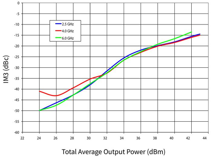
Figure 9. IM3 vs Total Average Power as a Function of Frequency
