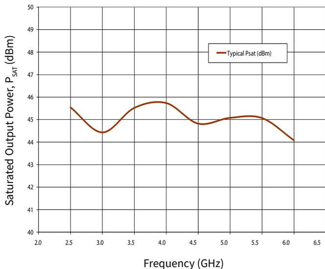
Figure 5. Saturated Output Power Performance (P<sub>SAT</sub>) vs Frequency
