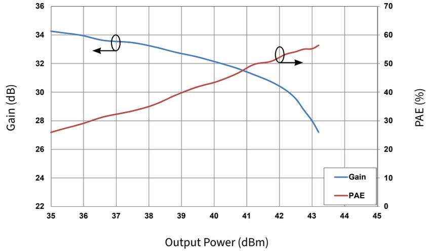
Figure 3. Gain and Power Added Efficiency vs Output Power Measured in CMPA2735015S-AMP1 Amplifier Circuit
