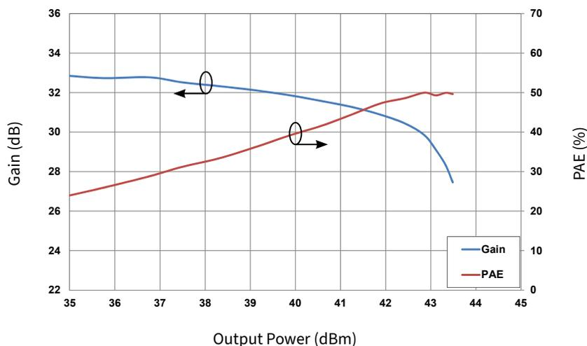
Figure 5. Gain and Power Added Efficiency vs Output Power Measured in CMPA2735015S-AMP1 Amplifier Circuit
