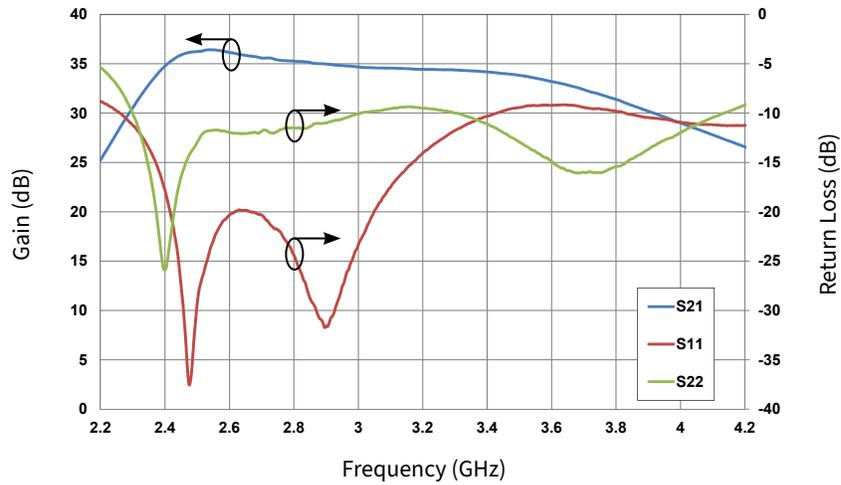
Figure 1. Gain and Return Loss vs Frequency of the CMPA2735015S Measured in CMPA2735015S-AMP1 Amplifier Circuit
