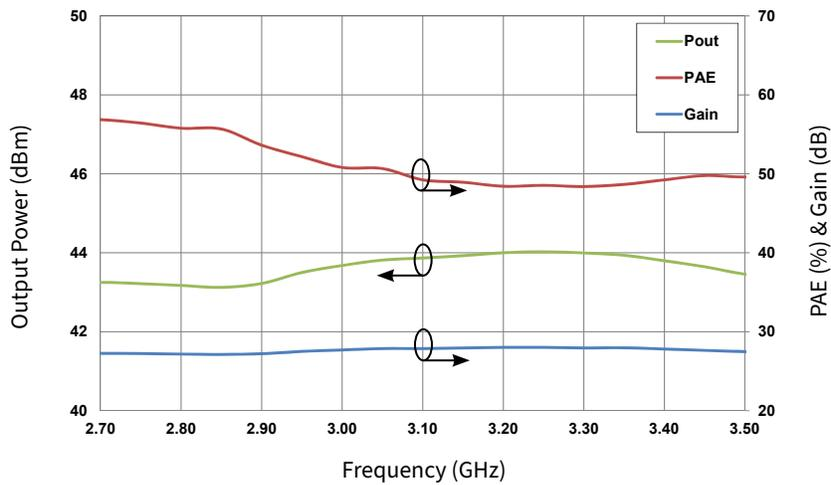
Figure 2. Output Power, Gain and PAE vs Frequency of the CMPA2735015S Measured in CMPA2735015S-AMP1 Amplifier Circuit
