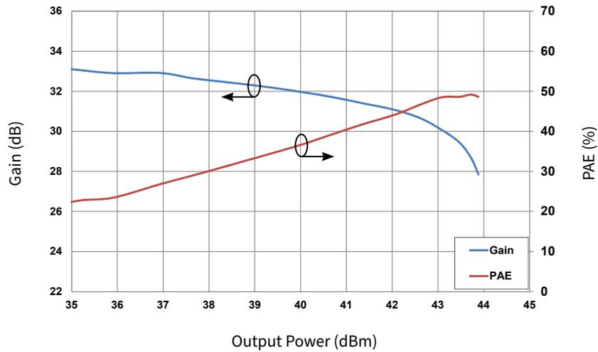
Figure 4. Gain and Power Added Efficiency vs Output Power Measured in CMPA2735015S-AMP1 Amplifier Circuit
