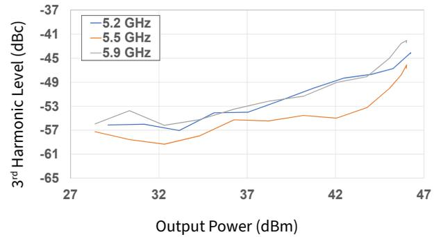
Figure 31. 3<sup>rd</sup> Harmonic vs Output Power as a Function of Frequency
