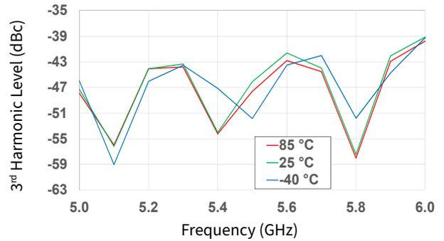
Figure 29. 3<sup>rd</sup> Harmonic vs Frequency as a Function of Temperature
