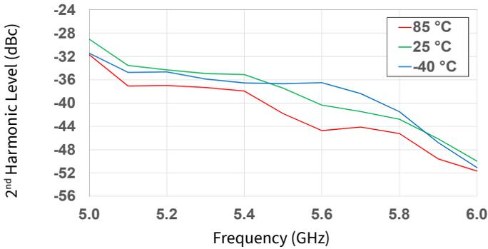
Figure 28. 2<sup>nd</sup> Harmonic vs Frequency as a Function of Temperature
