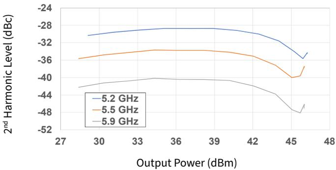
Figure 30. 2<sup>nd</sup> Harmonic vs Output Power as a Function of Frequency
