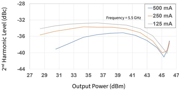
Figure 32. 2<sup>nd</sup> Harmonic vs Output Power as a Function of  $I_{DQ}$
