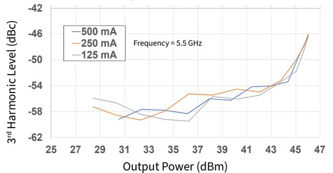
Figure 33. 3<sup>rd</sup> Harmonic vs Output Power as a Function of  $I_{DQ}$
