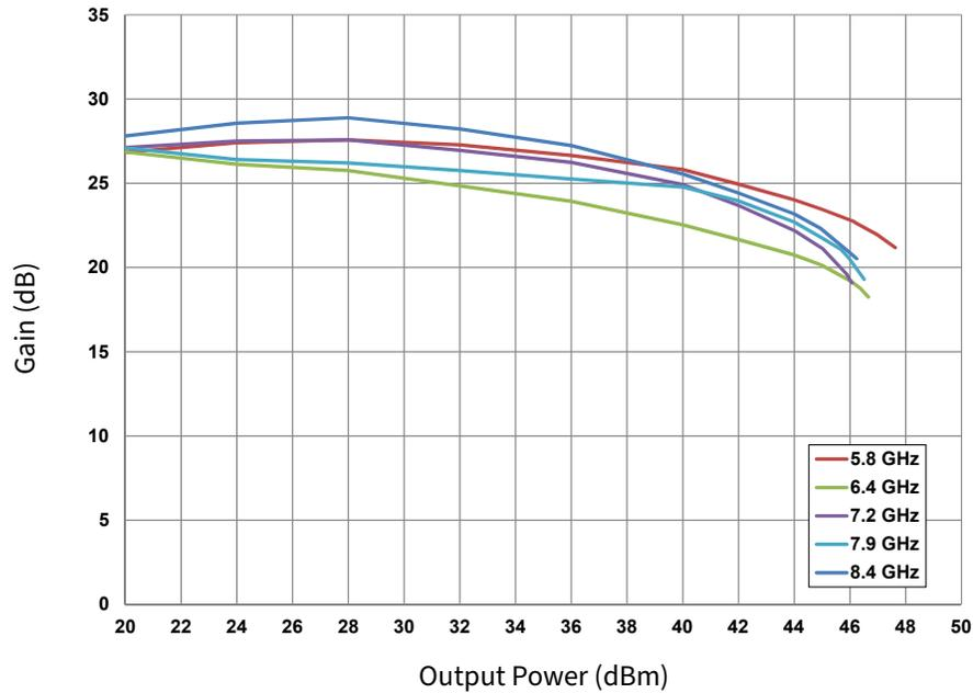
**Figure 12.** Gain vs. Output Power and Frequency
