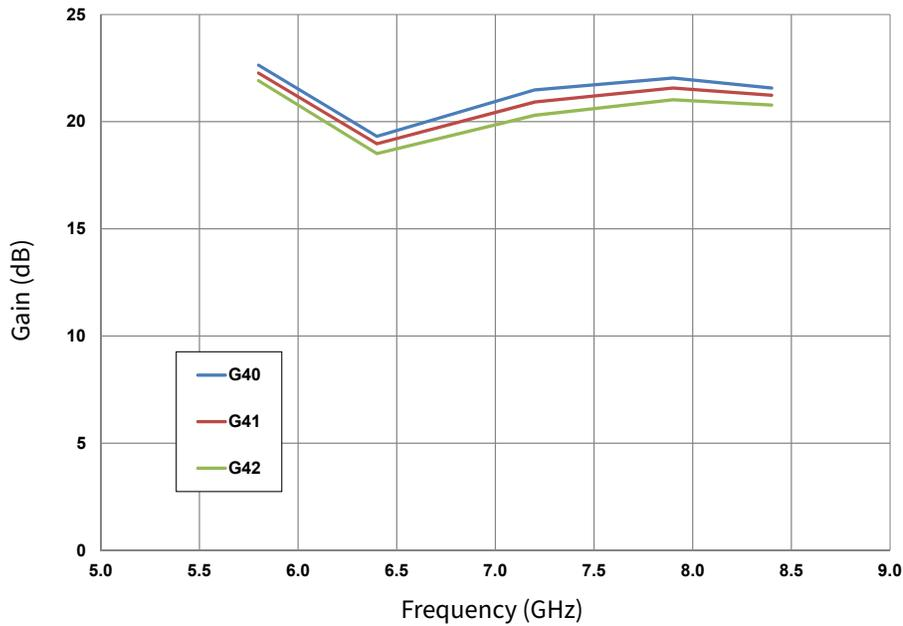
**Figure 1.** Gain vs. Frequency & Output Power OQPSK 1.6 Msps
