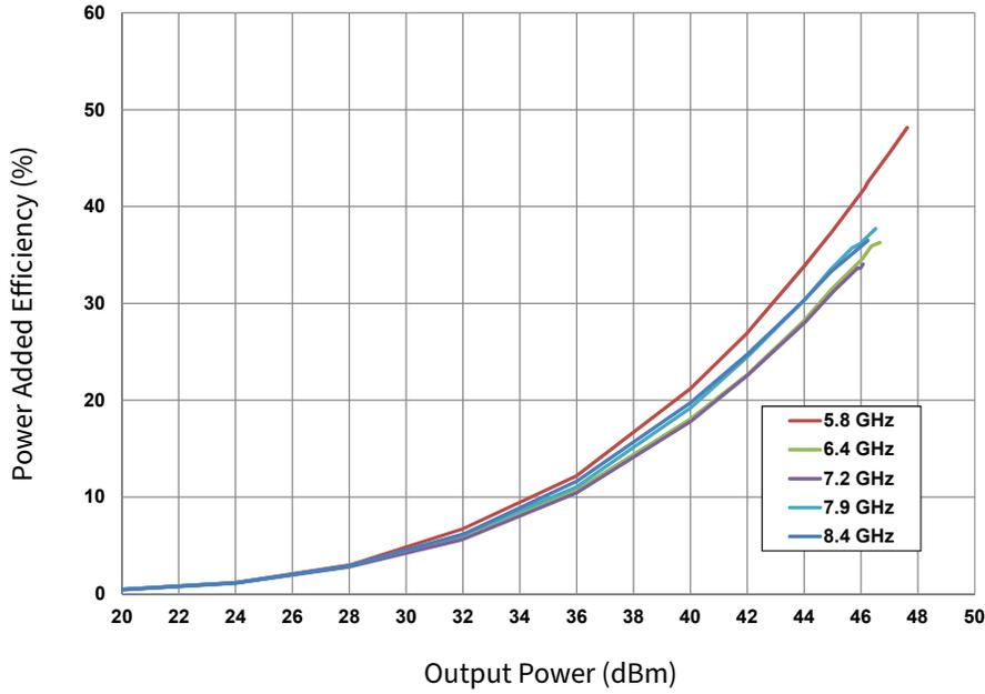
**Figure 11.** PAE vs. Output Power and Frequency
