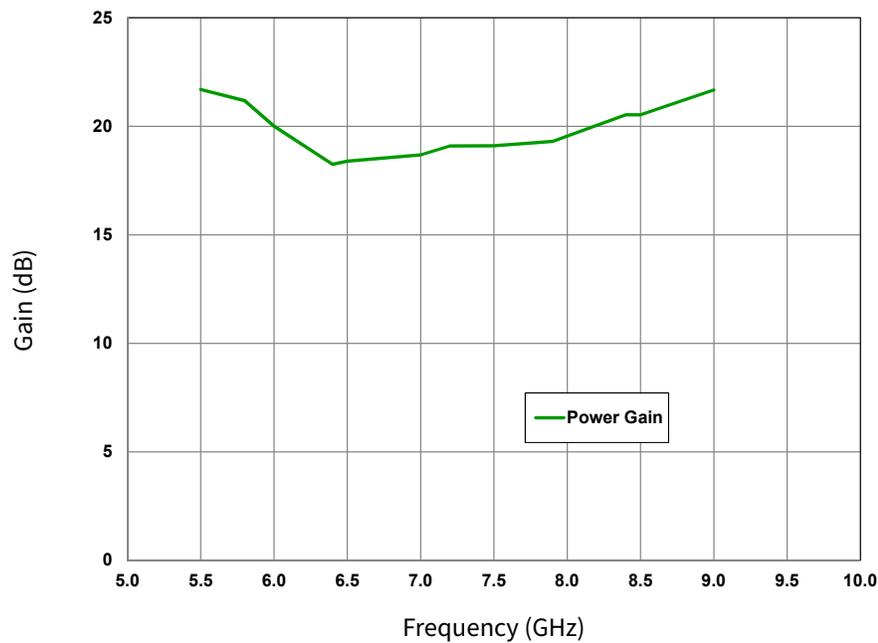
**Figure 10.** Gain @ Saturated Power vs. Frequency
