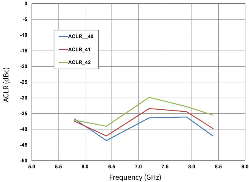
**Figure 3.** ACLR vs. Frequency & Output Power OQPSK 1.6 Msps
