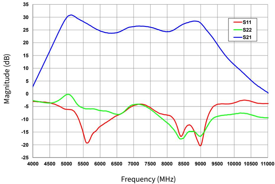
**Figure 4.** Typical S-Parameters
