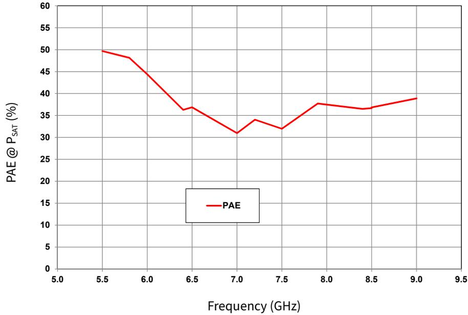
**Figure 9.** Power Added Efficiency @ Saturated Power vs. Frequency
