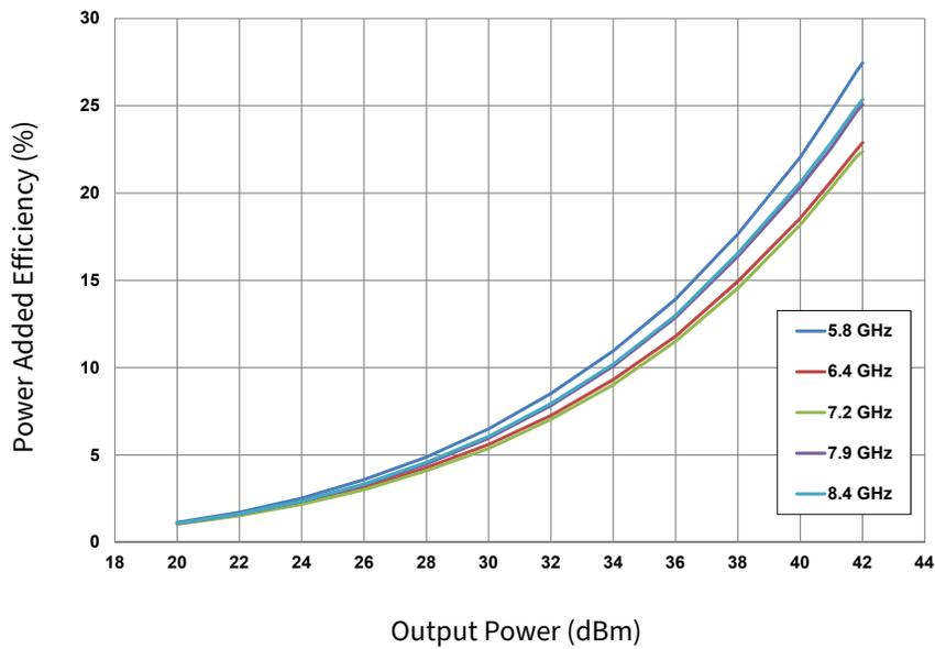
**Figure 6.** Power Added Efficiency vs. Output Power and Frequency OQPSK
