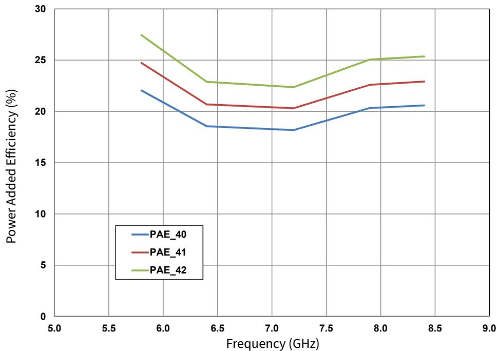
**Figure 2.** Power Added Efficiency vs. Frequency & Output Power OQPSK
