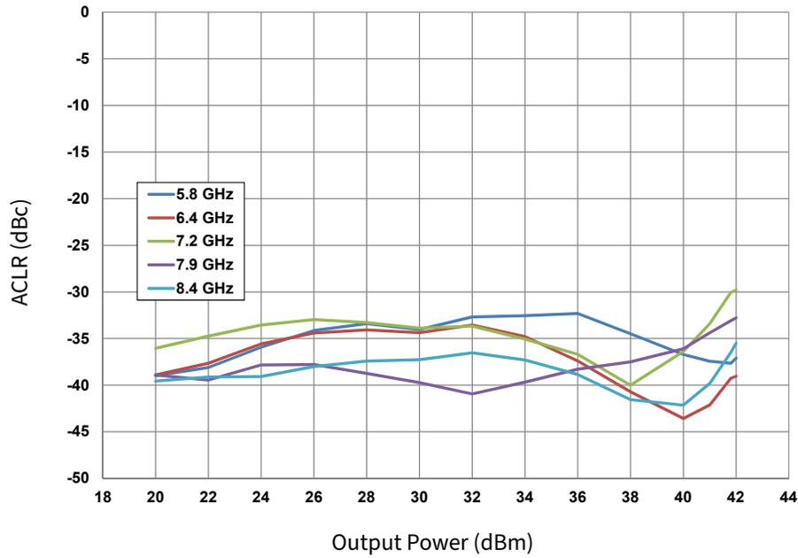
**Figure 7.** ACLR vs. Output Power and Frequency OQPSK 1.6 Msps
