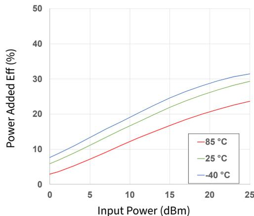
Figure 64. Power Added Eff. vs Input Power as a Function of Temperature
