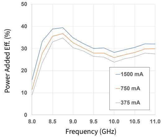
Figure 54. Power Added Eff. vs Frequency as a Function of  $I_{DQ}$
