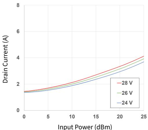
Figure 70. Drain Current vs Input Power as a Function of Voltage
