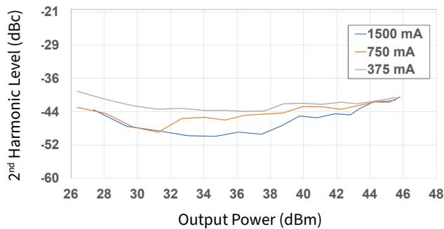
Figure 30. 2<sup>nd</sup> Harmonic vs Output Power as a Function of  $I_{DQ}$
