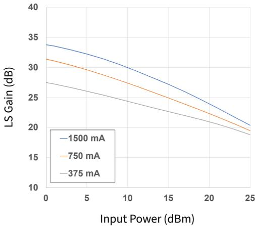
Figure 77. Large Signal Gain vs Input Power as a Function of  $I_{DQ}$
