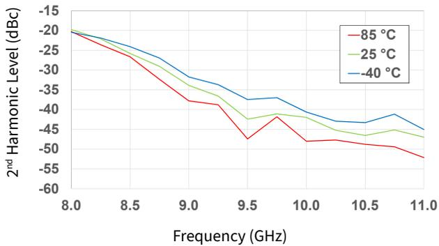
Figure 28. 2<sup>nd</sup> Harmonic vs Frequency as a Function of Temperature
