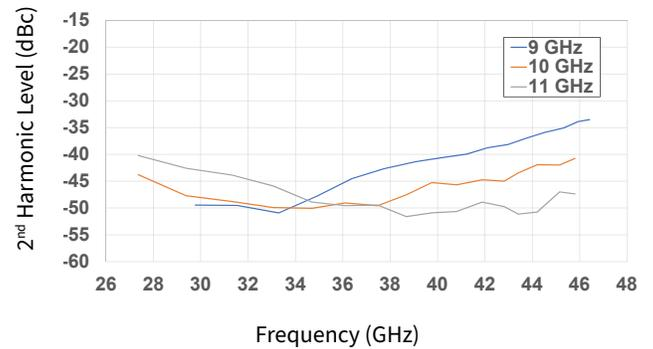
Figure 29. 2<sup>nd</sup> Harmonic vs Output Power as a Function of Frequency
