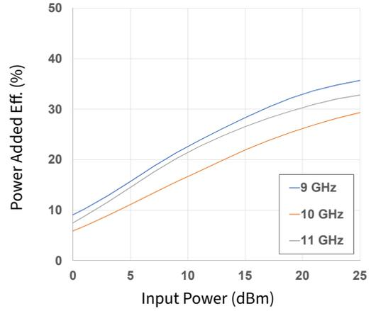
Figure 59. Power Added Eff. vs Input Power as a Function of Frequency
