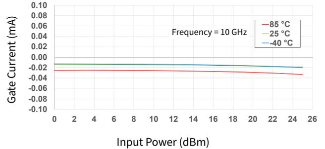
Figure 22. Gate Current vs Input Power as a Function of Temperature
