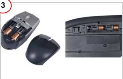
Power the mouse and keyboard with two AA batteries each.
