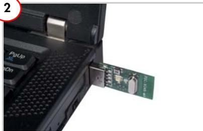
Connect the bridge dongle to the PC. The bridge enumerates as a human interface device (HID).
