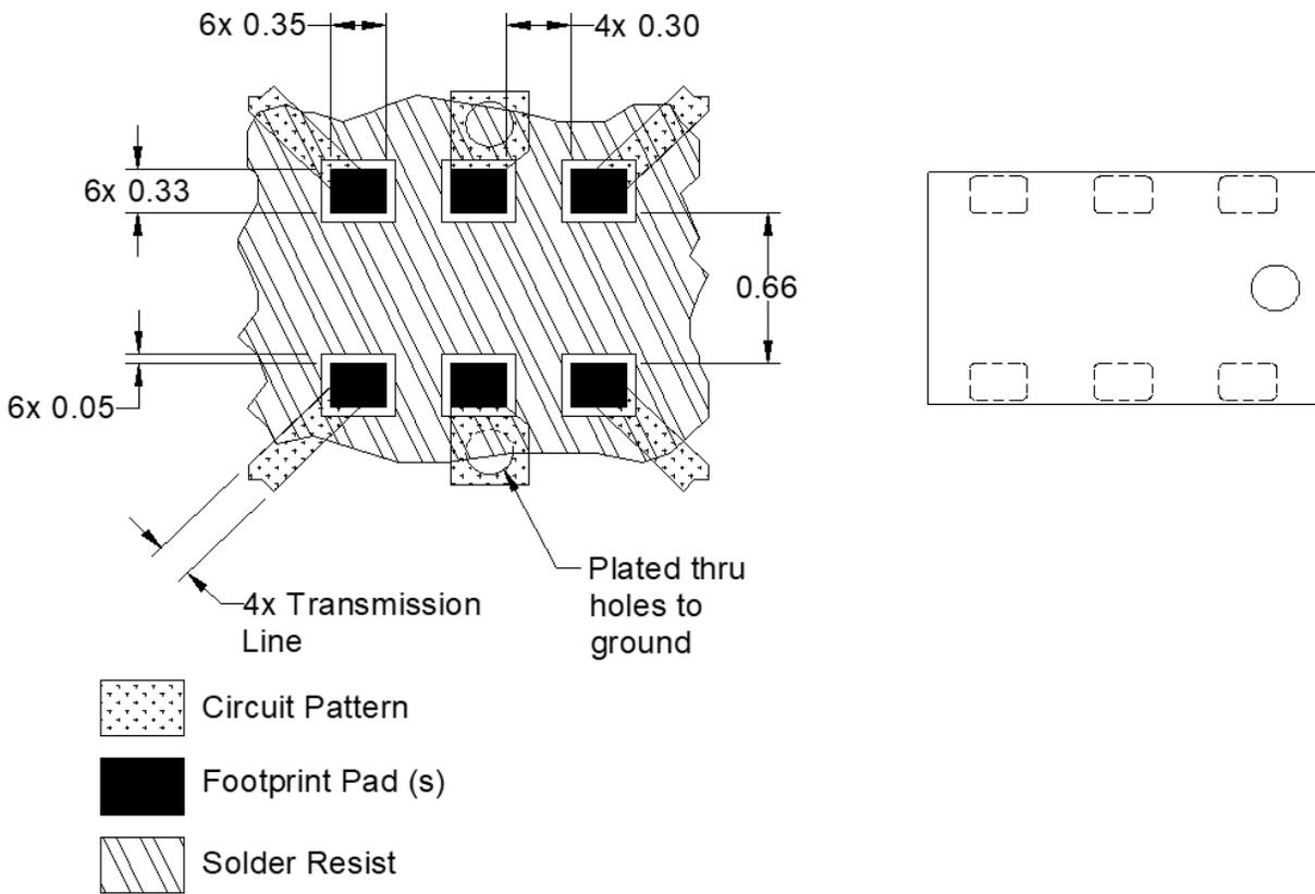
Dimensions are in Millimeters
