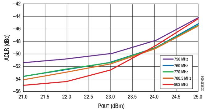
Figure 6. ACLR (5 MHz) vs POUT Across Frequency
