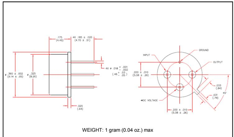
\* Dimensions are inches (millimeters)  $\pm 0.015$  (0.38) unless otherwise specified.
