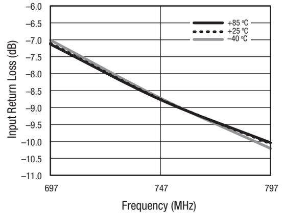
Figure 6. Input Return Loss vs Frequency Over Temperature
