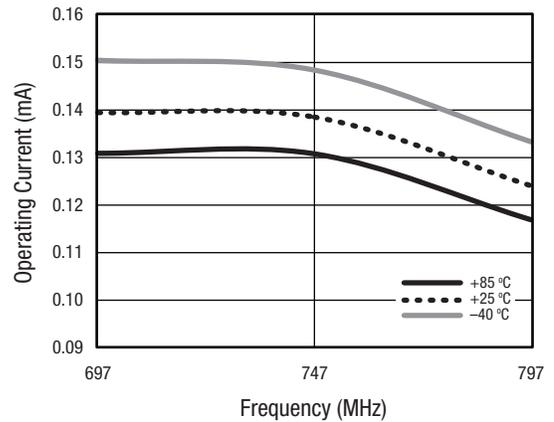
Figure 30. Operating Current @ P1dB vs Frequency Over Temperature
