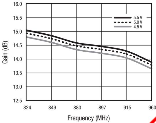
Figure 36. Small Signal Gain vs Frequency Over VCC
