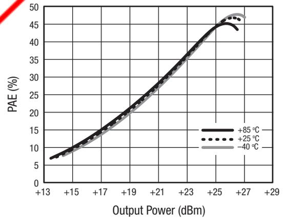
Figure 55. PAE vs Output Power Over Temperature
