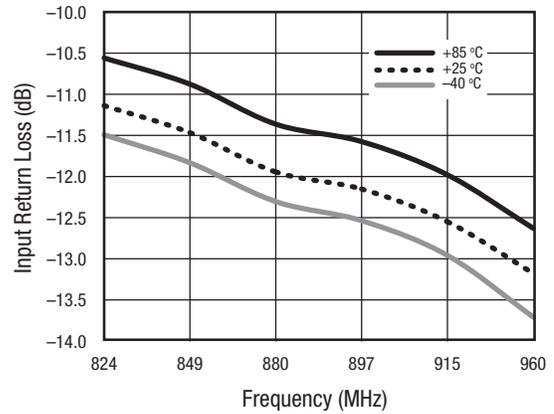
Figure 39. Input Return Loss vs Frequency Over Temperature
