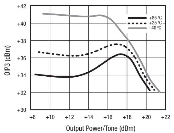
Figure 51. OIP3 vs Output Power/Tone Over Temperature
