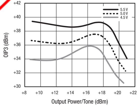
Figure 49. OIP3 vs Output Power/Tone Over VCC
