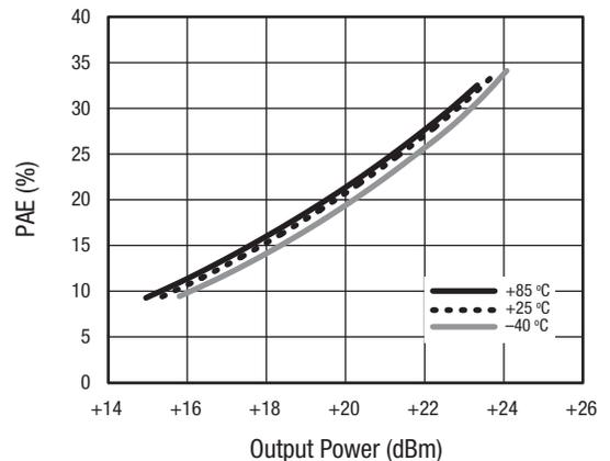
Figure 18. PAE vs Output Power Over Temperature
