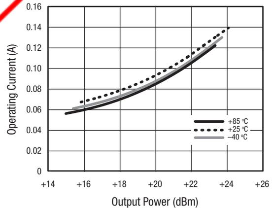
Figure 34. Operating Current vs Output Power Over Temperature
