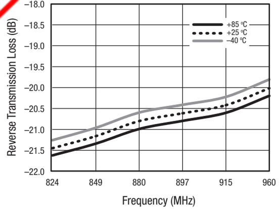
Figure 43. Reverse Transmission Loss vs Frequency Over Temperature
