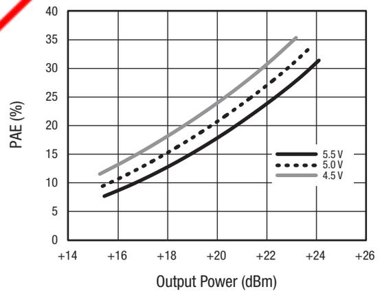
Figure 16. PAE vs Output Power Over VCC
