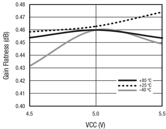
Figure 31. Gain Flatness vs VCC Over Temperature
