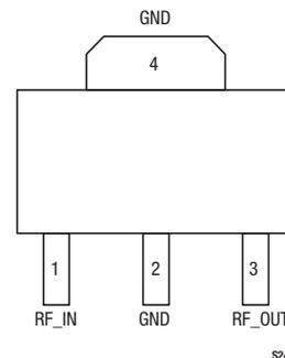
Figure 1. SKY65045-70LF Pinout Package (Top View)
