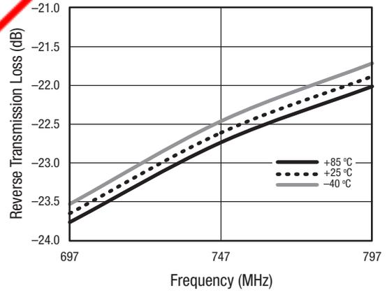
Figure 10. Reverse Transmission Loss vs Frequency Over Temperature
