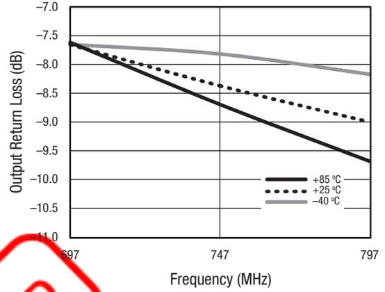
Figure 8. Output Return Loss vs Frequency Over Temperature
