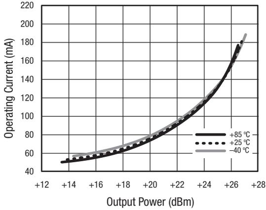
Figure 58. Operating Current vs Output Power Over Temperature
