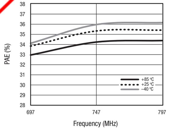
Figure 28. PAE @ P1dB vs Frequency Over Temperature
