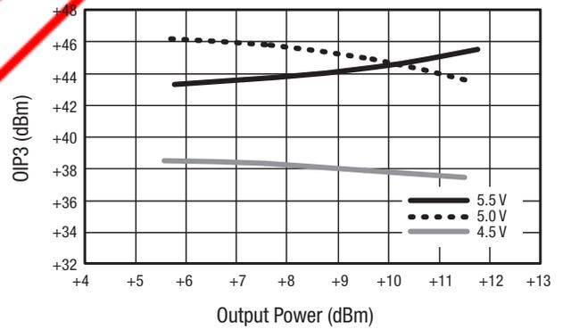
Figure 22. OIP3 vs Output Power Over VCC
