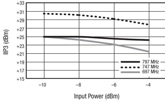
Figure 25. IIP3 vs Input Power Over Frequency
