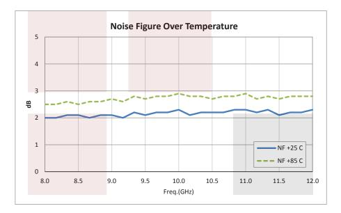
2.2 dB NF Low Noise Amplifier Operating From 8 GHz to 12 GHz with 28 dB Gain, 13 dBm Psat and SMA from Fairview Microwave is in-stock and available to ship same-day. All of our RF/microwave products are available off-the-shelf from our ISO 9001:2008 certified facilities in Allen, Texas. Fairview Microwave is RF on-demand.
