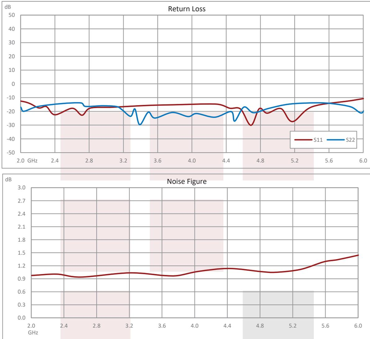
1.2 dB NF Input Protected Low Noise Amplifier, Operating from 2 GHz to 6 GHz with 40 dB Gain, 14 dBm P1dB and SMA from Fairview Microwave is in-stock and available to ship same-day. All of our RF/microwave products are available off-the-shelf from our ISO 9001:2008 certified facilities in Lewisville, Texas. Fairview Microwave is RF on-demand.
